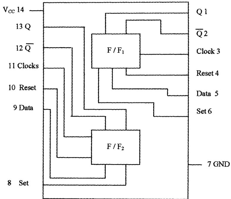
Fig 3.3 Pin Assignment of 4013B
