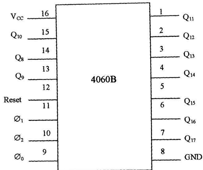
Fig 3.2 Pin Assignment of 4060B
