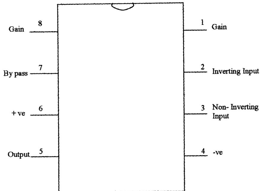
Fig 3.6 Pin assignment of LM 386
