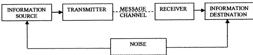
Fig 2.3 A Basic Communication Model
