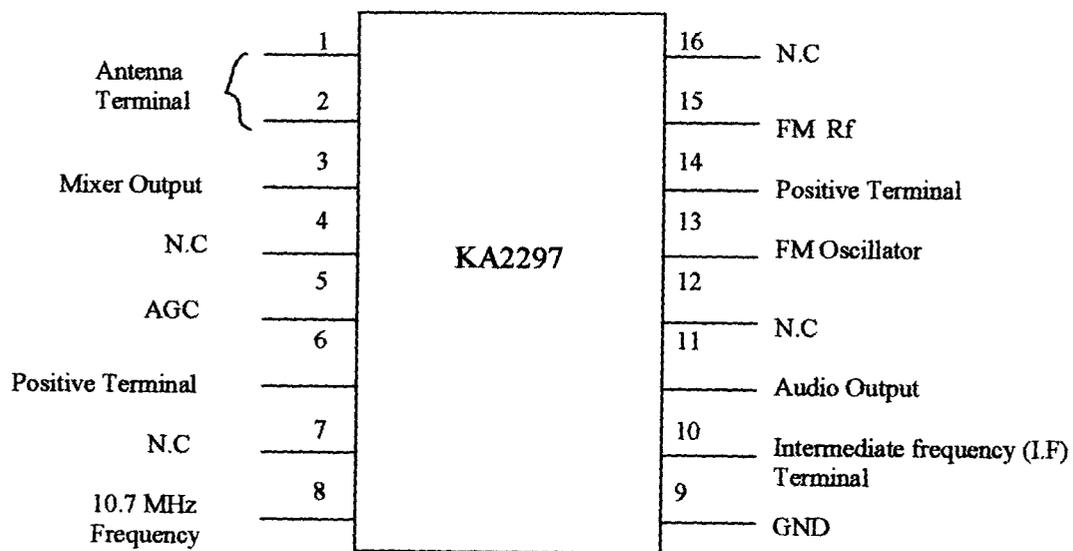
Fig 3.4 Pin Connection of KA2297
