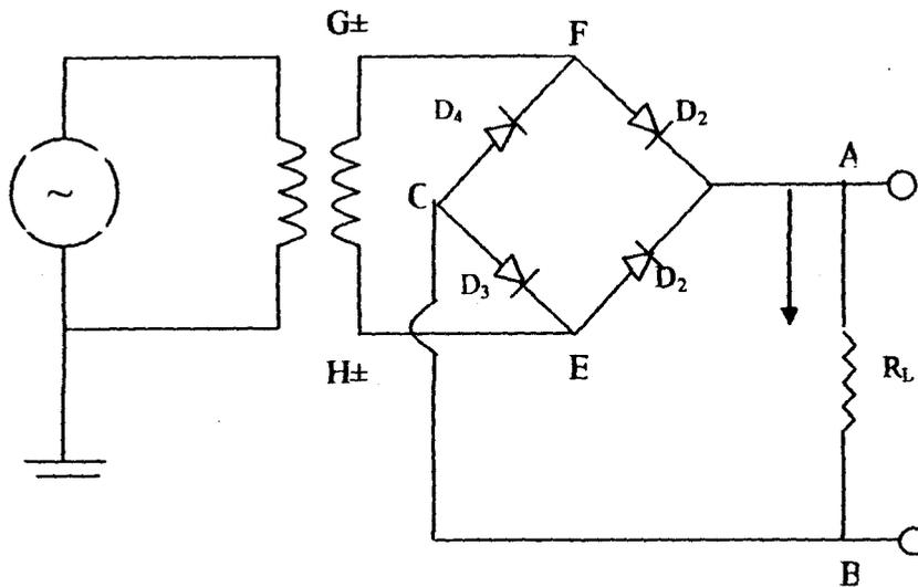
Fig. 3.4 Full-wave rectifier circuit using diodes
