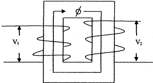
Fig. 3.3 Primary and secondary winding of transformer
