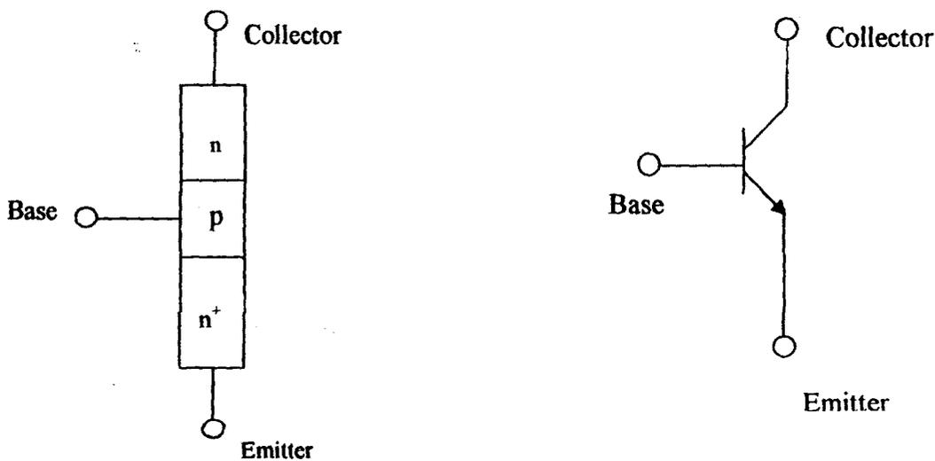
Fig. 3.5a npn transistor
