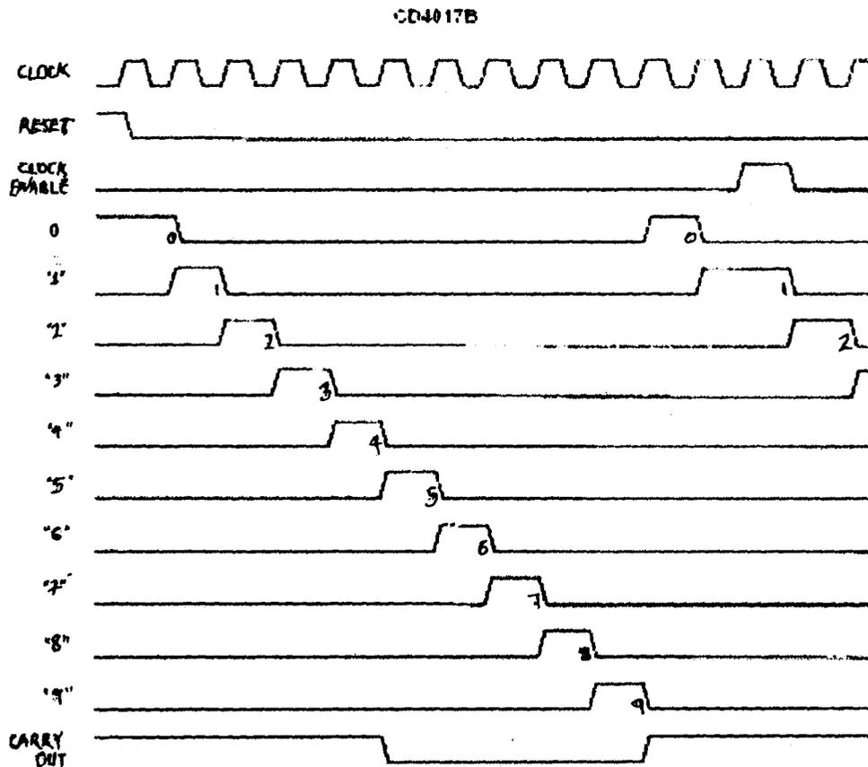
Fig. 3.5.6: Pin assignment and timing diagram of 4017B IC
