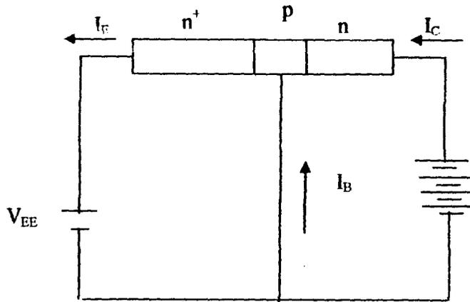
Fig. 3.5.1 Biasing of npn transistor
