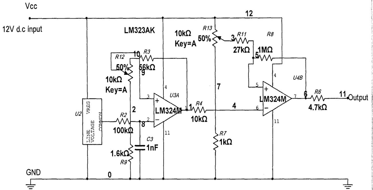
Fig: 3.8 Schematic diagram of a sensing circuit
