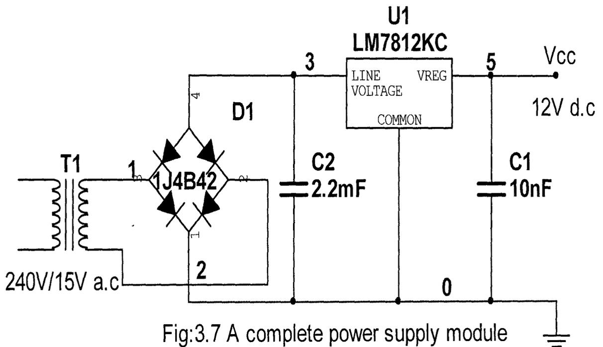
Fig:3.7 A complete power supply module
