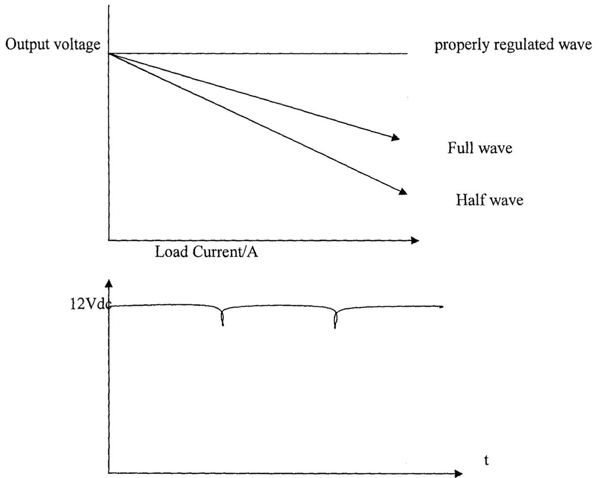
**Fig 3.6 wave forms of regulated voltage output**
