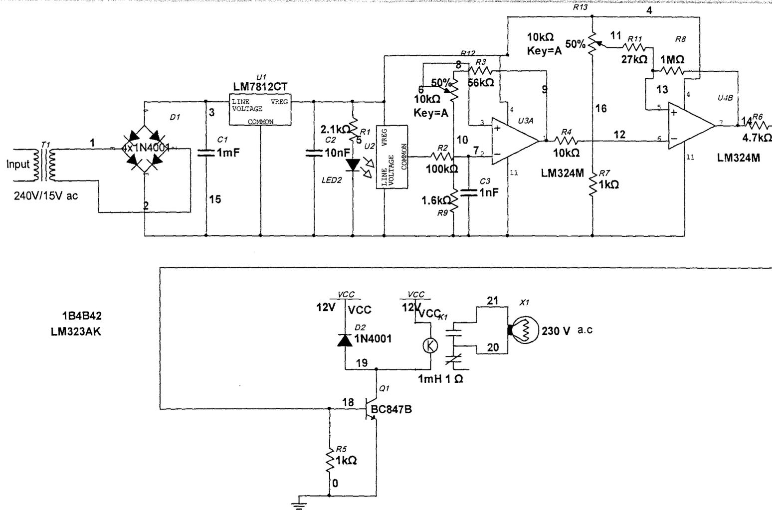
Figure: 4.0 A COMPLETE CIRCUIT DIAGRAM OF AN AUTOMATIC ROOM CONTROLLED HEATING SYSTEM
