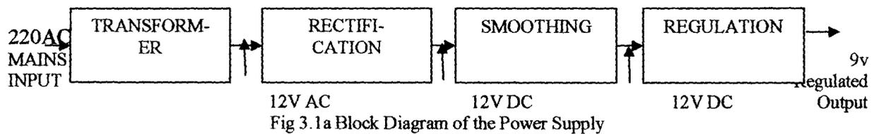
The circuit diagram for the power supply is shown in figure 3.1b. An important characteristic of this diagram is the use of 7809 regulator chip. This chip provides the output that is needed to power the system properly.
