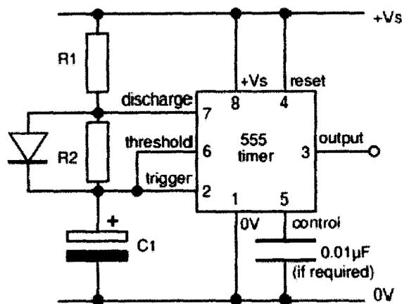
FIG 3.4 555 astable circuit with diode across R2
