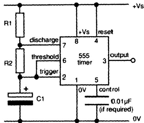
FIG 3.3 555 astable circuit
