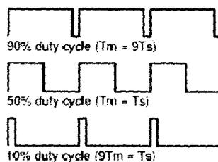
For a standard 555/556 astable circuit the mark time ( $T_m$ ) must be greater than the space time ( $T_s$ ), so the duty cycle must be at least 50%:
