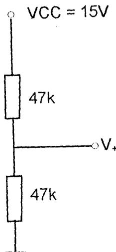
Fig. 3.4 showing the biasing arrangement of the pre-amplifier stage.
