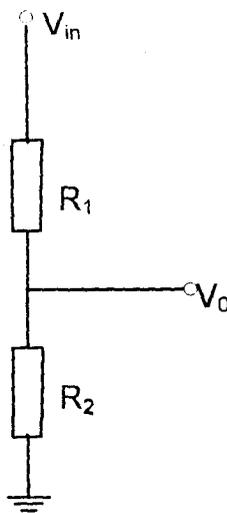
Fig 3.5 showing biasing arrangement.
