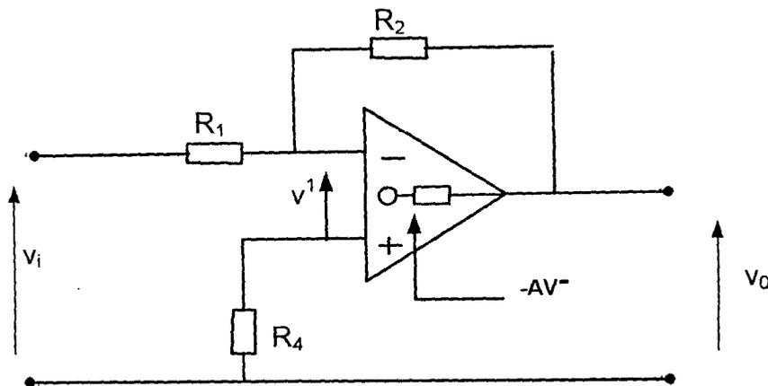
Fig. 2.5 Input and output impedance of an inverting amplifier.
