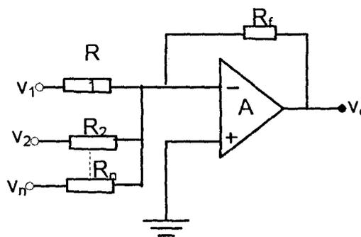
Fig 2.10 Showing op-amp as an adder or summing amplifier.
