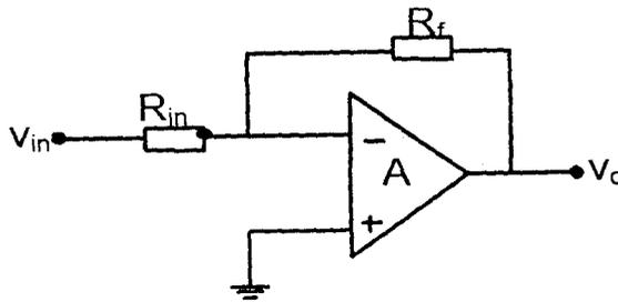
Fig. 2.7 Showing an operational amplifier as a sign changer.
