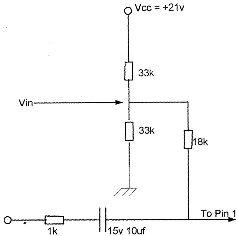
Fig. 3.8 showing the biasing arrangement.
