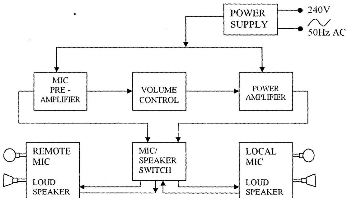
Fig 1.1 BLOCK DIAGRAM OF A SINGLE CHANNEL INTERCOM SYSTEM
