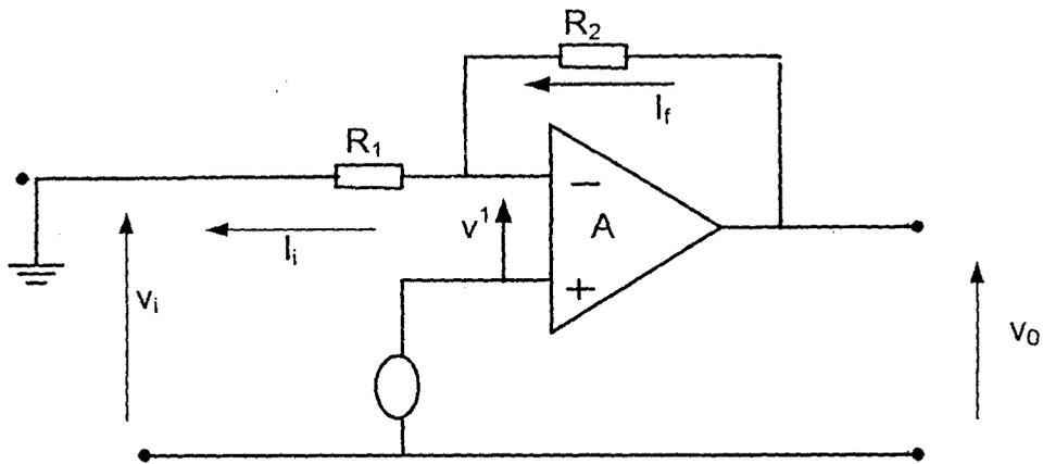
Fig. 2.6 Showing non – inverting operational amplifier connection.
