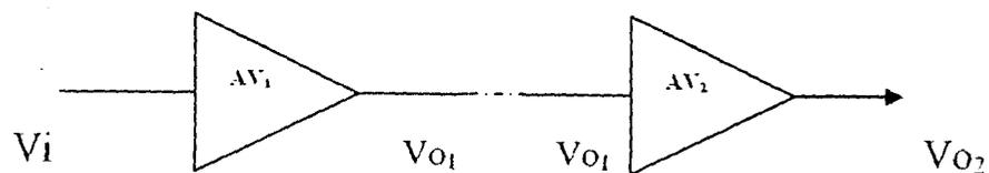
Fig. 2.2 Showing Amplifier in series.
