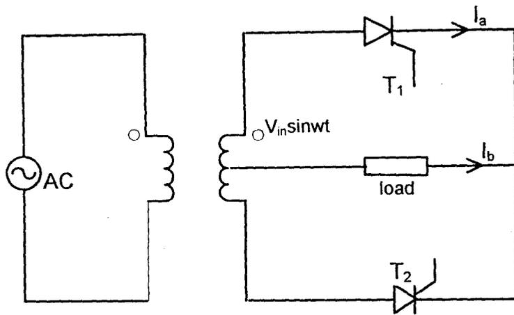
Fig. 2.12b Show a Bi-phase full wave connection.
