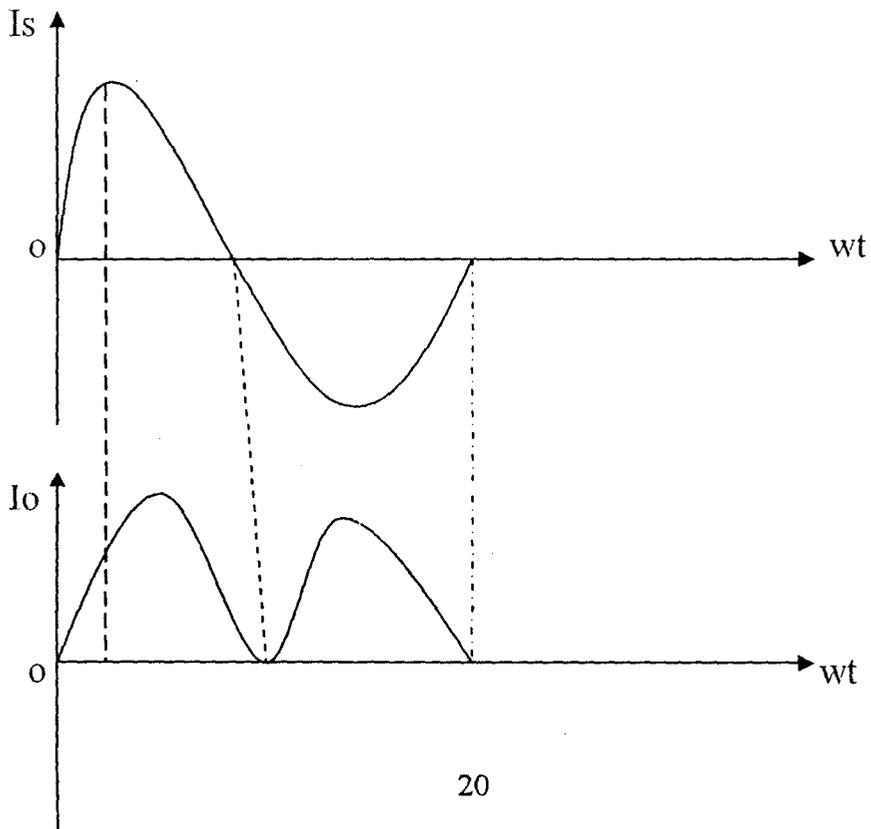
Fig. 2.12d showing the output wave forms of a full wave rectifier.
