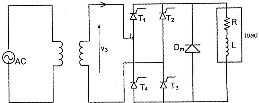
Fig 2.13a Shows a Bridge Converter Circuit.
