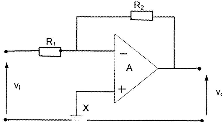
Fig. 2.3 Inverting operational amplifier.
