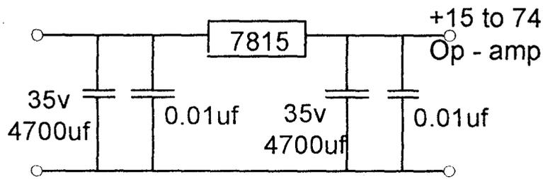
Fig. 3.2 Showing regulation unit connections.
