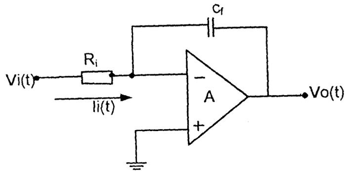
Fig. 2.8 showing op-amp as an integrator.
