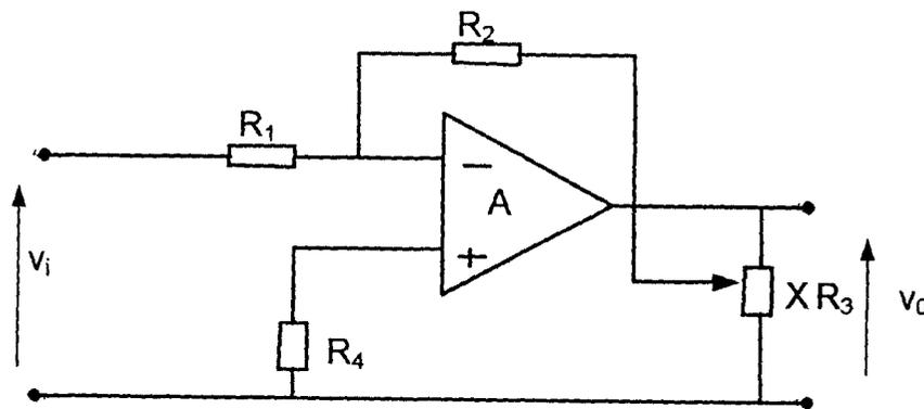
Fig. 2.4 showing the gain of the inverting amplifier.
