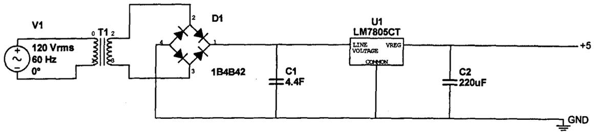
fig. 3.2 circuit diagram of power supply unit
