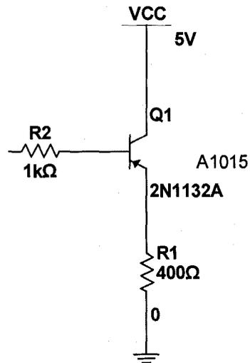
Fig. 3.3 Design of relay driver
