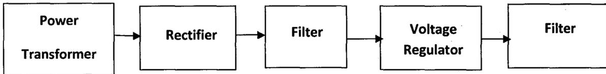
Fig 3.1 Block Diagram of Power Supply Unit
