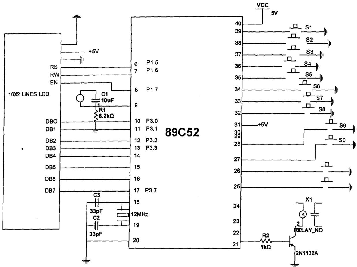
Fig 3.4 Circuit diagram showing the design and construction of an electronic timed mosquito fleeing system
