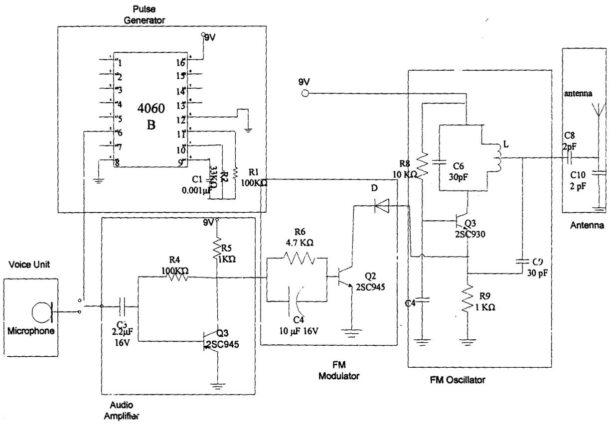
fig 3.4.i.2 The Transmitter Circuit Diagram
