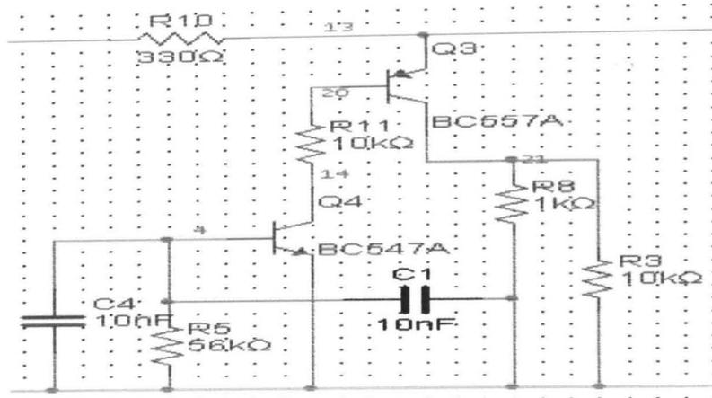
Fig. 8: voltage controlled oscillator of the circuit
