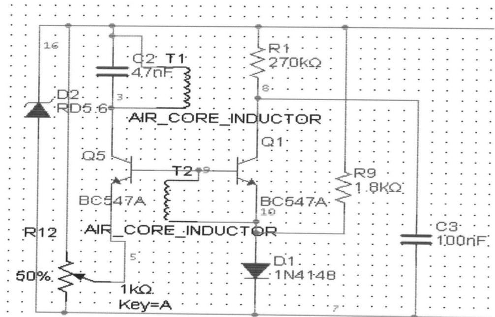
Fig. 7: Feedback oscillator of the circuit
