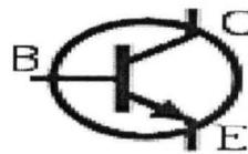
Fig. 4: Symbol of a transistor
