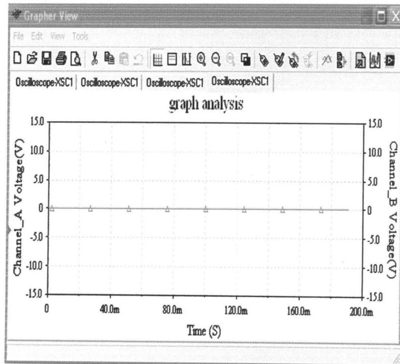
Plate VIII: Wave form when the buzzer does not produce sound
