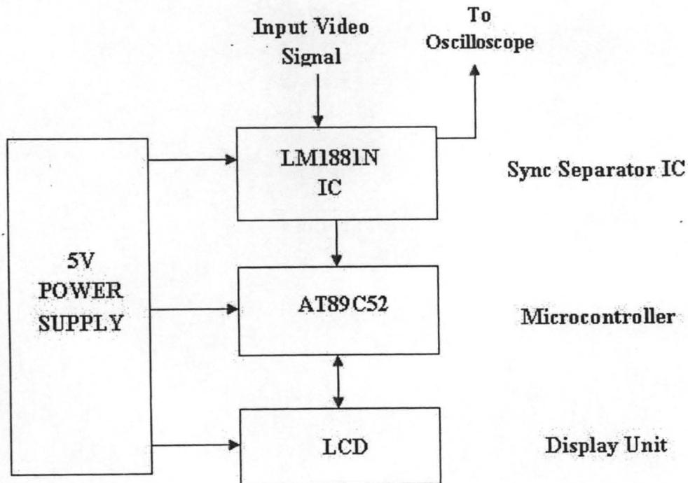
Figure 3.1: Block diagram of the Video Line Selector
