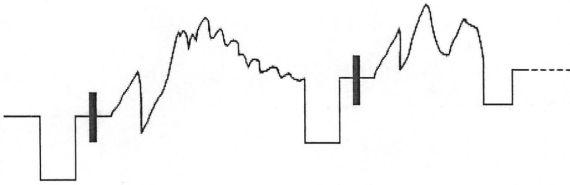
Figure 4.1 Output Video Si signal on LCD with video line connected
