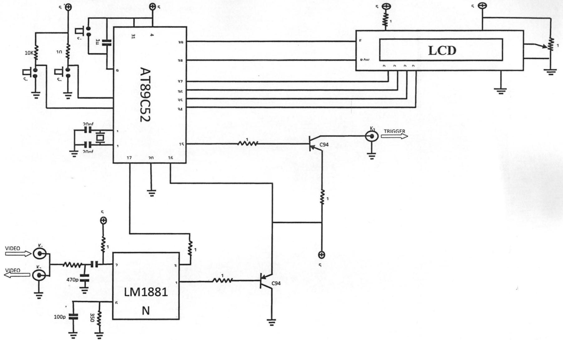
Figure 3.6: the complete circuit diagram of the Video Line Selector
