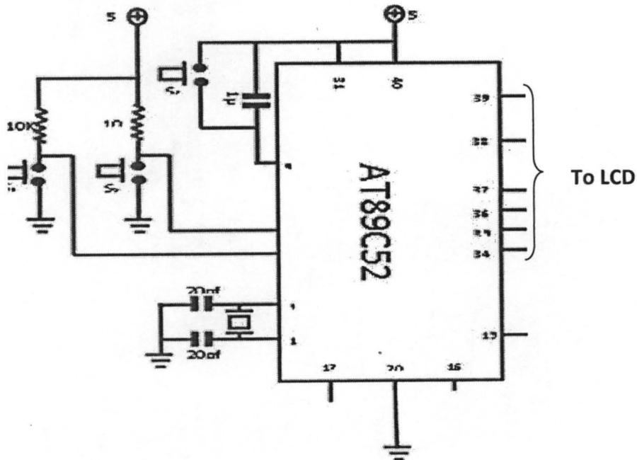
Figure 3.4: basic microcontroller pin configuration with interface indications
