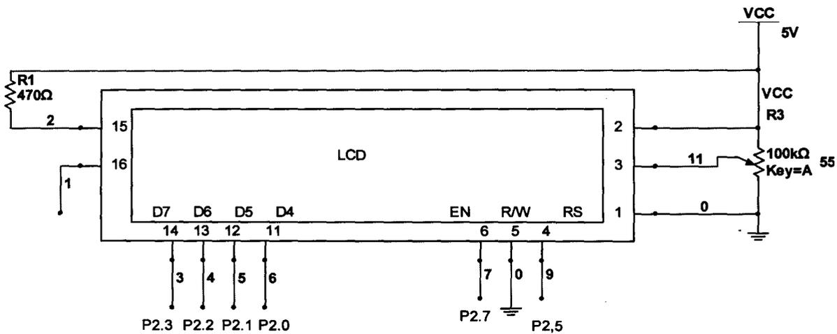
Figure 3.12: schematic diagram of display unit
