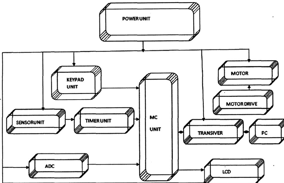
Fig 3.1: Solar tracker block diagram
