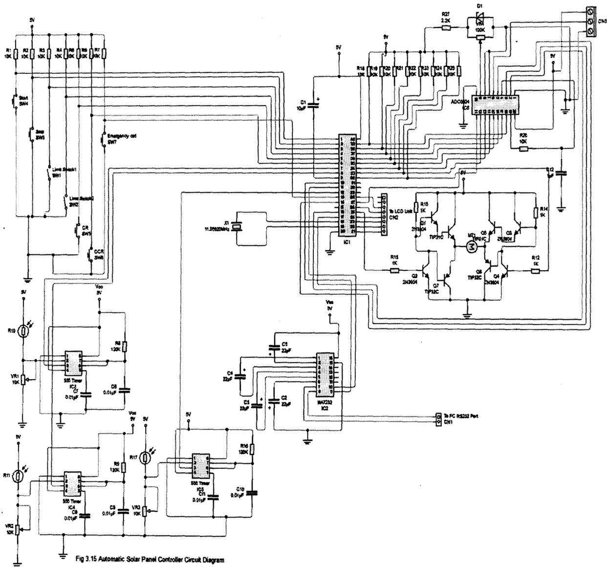
Fig 3.15 Automatic Solar Panel Controller Circuit Diagram
