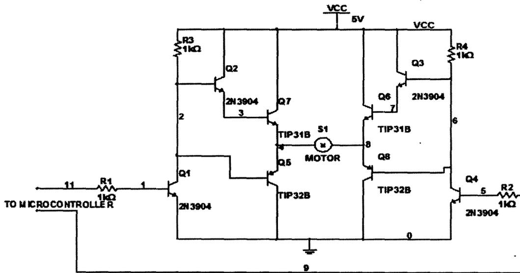
Figure 3.13: schematic diagram of motor unit
