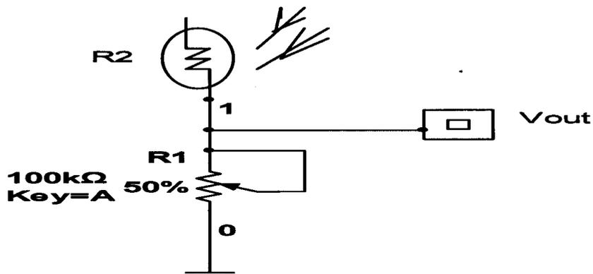
Fig.3.3: schematic diagram of solar sensing unit
