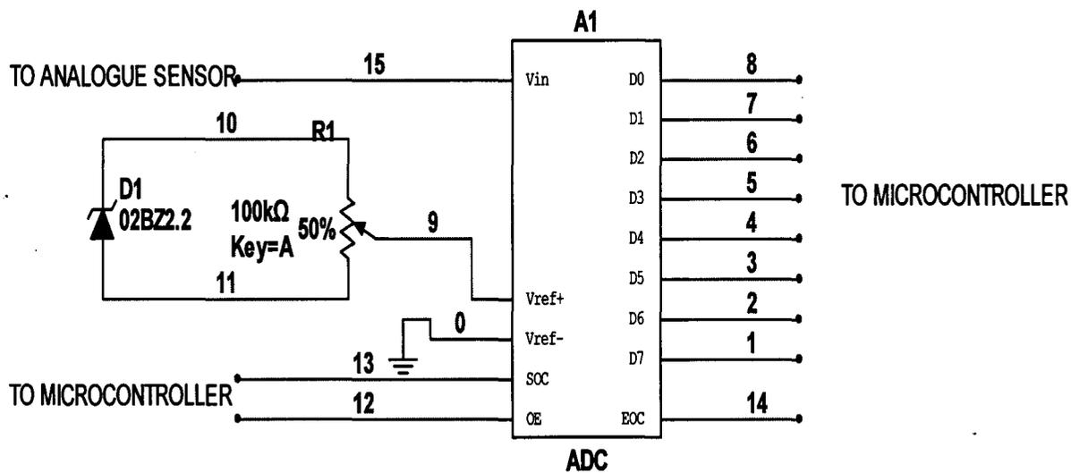
Fig.3.8: schematic circuit diagram of ADC unit
