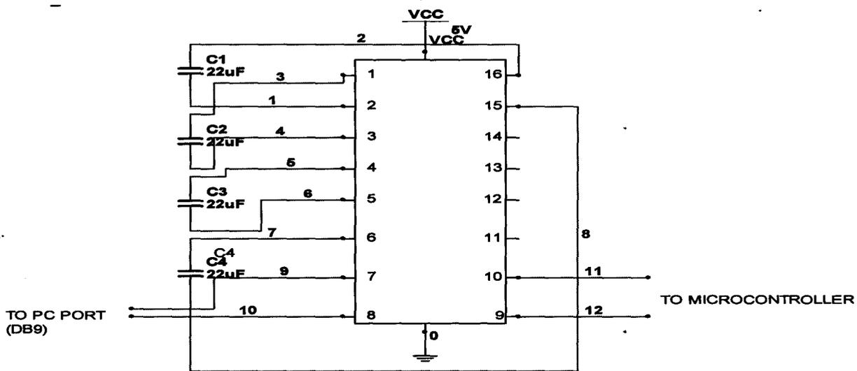
Figure 3.10: schematic diagram of transceiver unit
