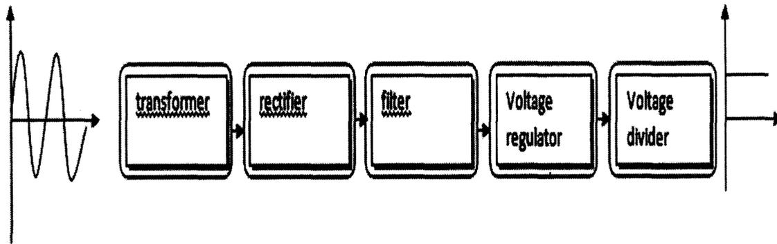
Figure:2.4 Block diagram of power unit
