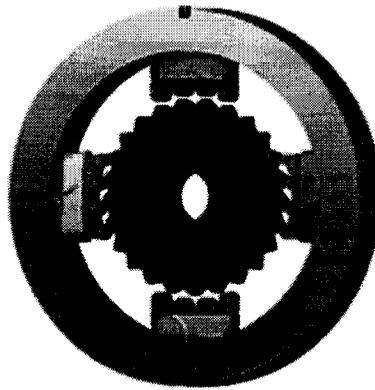
Figure:2. 1 Stepper motor
