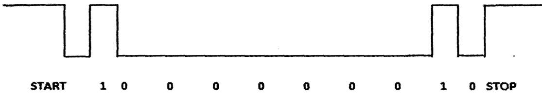
Fig.3.9: Bit pattern for transmitting character 'A'
