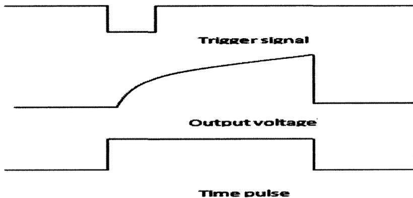
Fig. 3.7: Relationship between the trigger signal, the voltage on the capacitor and the pulse width in monostable mode
