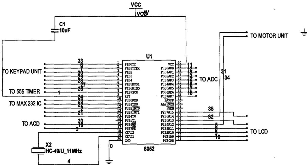
Fig.3.2: schematic circuit diagram of microcontroller unit
