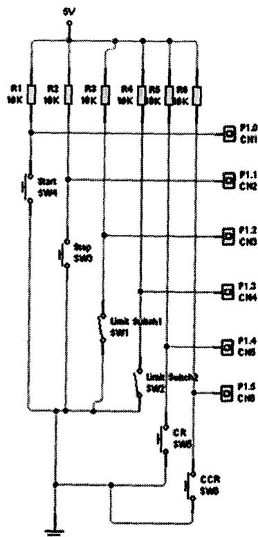
Figure 3.14: schematic diagram of keypad unit
