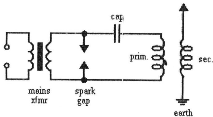
Fig 2.2 circuit diagram of a simple tesla coil
