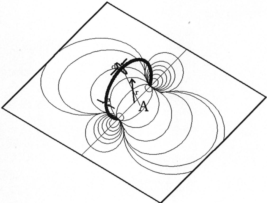
Fig 3.3 a capacitively loaded conducting wire loop
