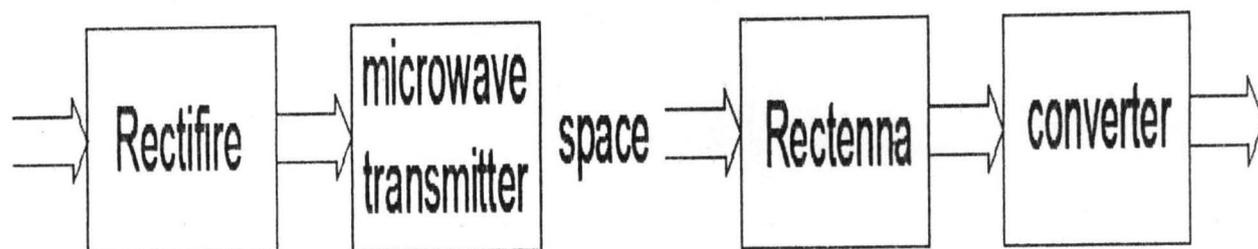
Fig 2.8 block diagram of microwave wireless power transmission
