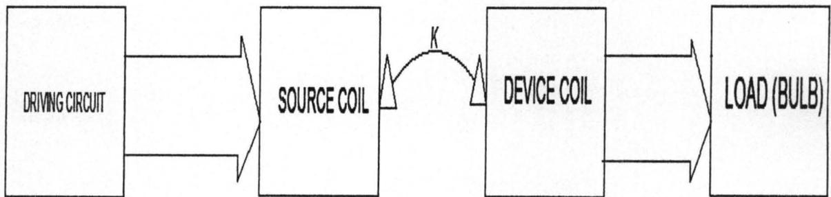
Fig 3.2 block diagram of the transfer scheme
