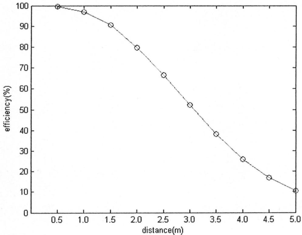
Fig 4.3 plot of efficiency against distance between loops
