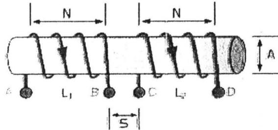
Fig 2.4 mutual inductance between two coils
