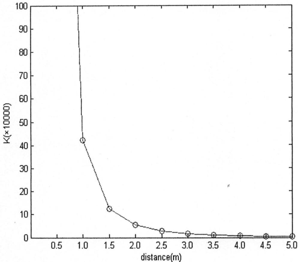
Fig 4.1 plot of coupling factor against distance between loop centers
