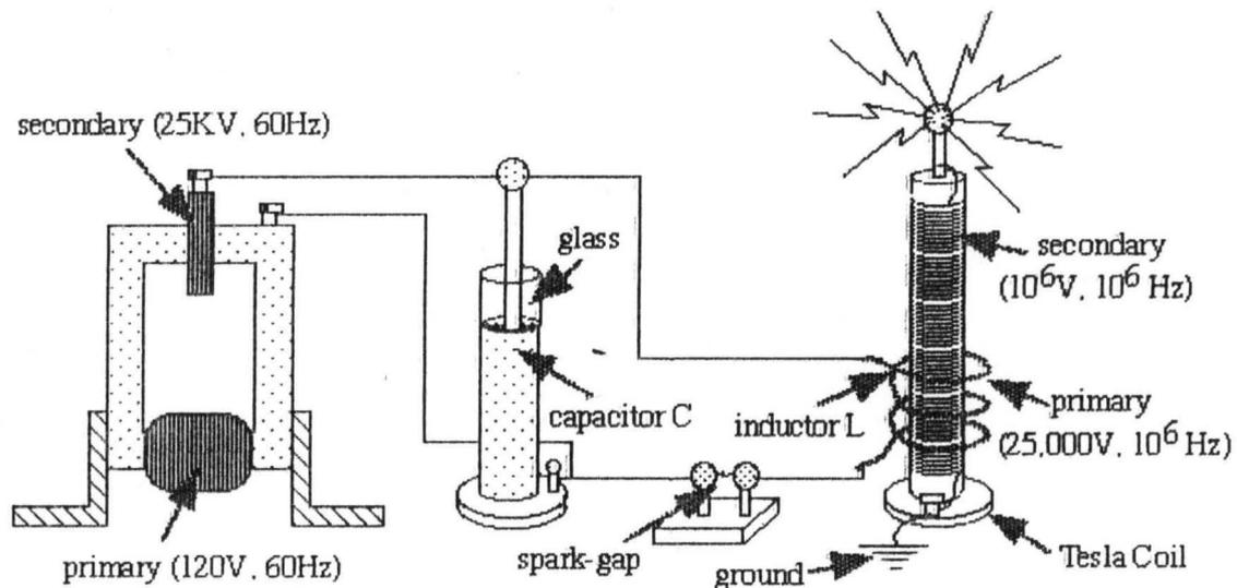
Fig 2.1 schematic diagram of a Tesla coil
