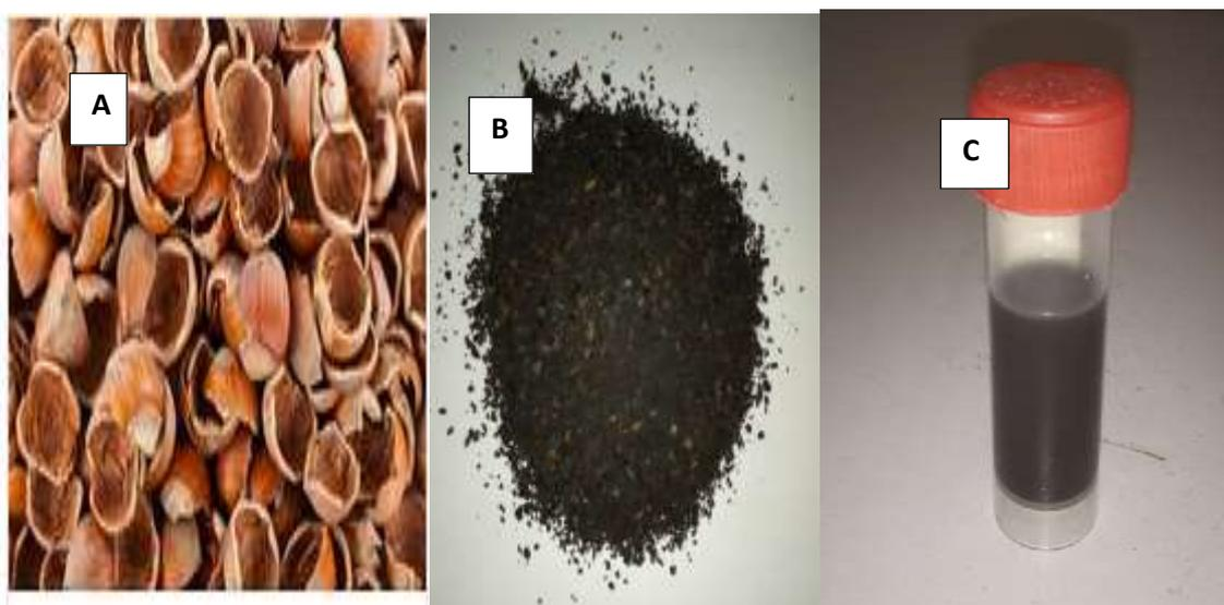
**PLATE I: (A) Shea butter shell (B) Bio-char (C) Bio-oil from fast pyrolysis**
