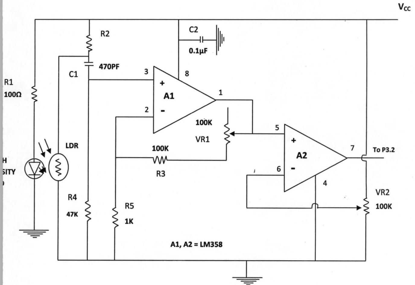
Figure 3.3 Heart Rate circuit diagram
