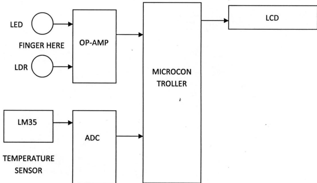
Fig. 3.1 block diagram of body temperature and heart beat monitoring device
