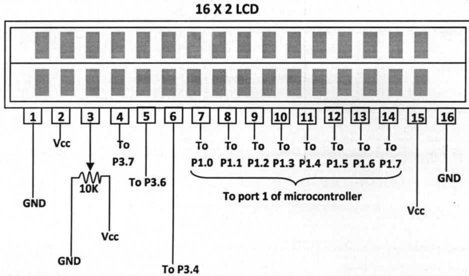
Figure 3.4 LCD pin configuration with microcontroller interface indications
