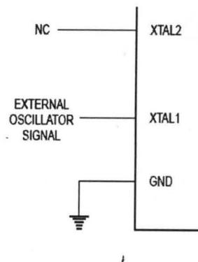
**Figure 2.3.external clock drive configuration**
