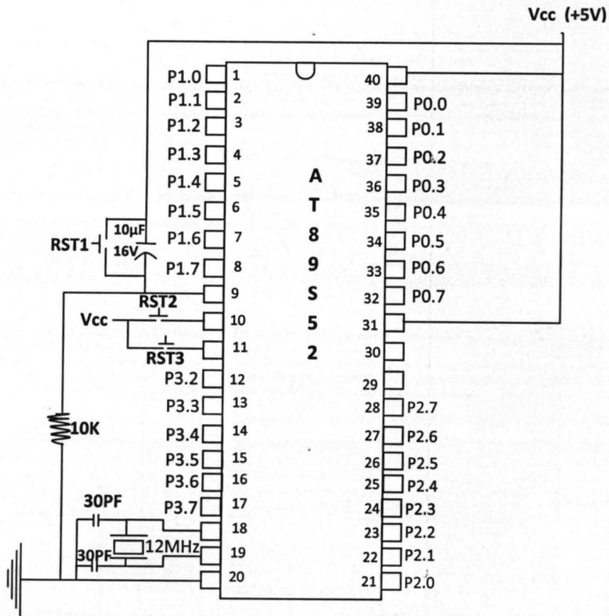
Figure 3.5 basic microcontroller pin configuration with interface indications
