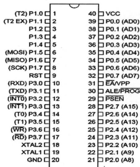
Figure 2.1 Diagram of AT89S52 microcontroller showing the pin configuration
