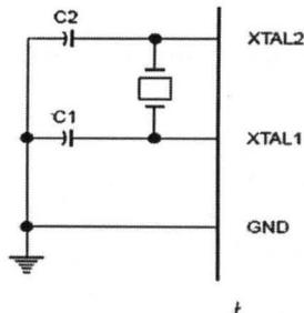
**Figure 2.2.oscilator connection**
