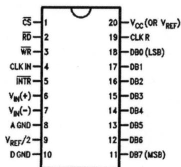
Fig. 1.0 Diagram of ADC0804 showing pin configuration
