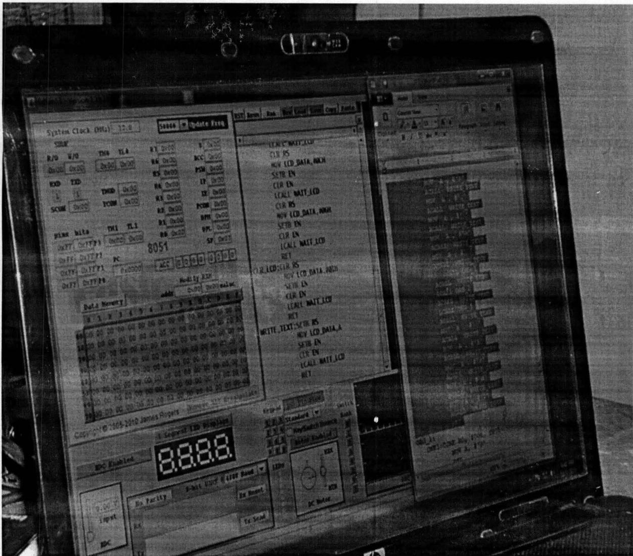
i. A screen-shot of the assembly code using *EdSim51* assembler
