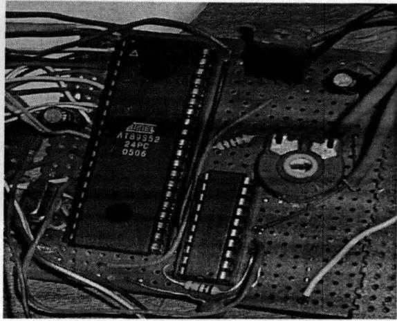
g. Temperature unit interfaced to microcontroller
