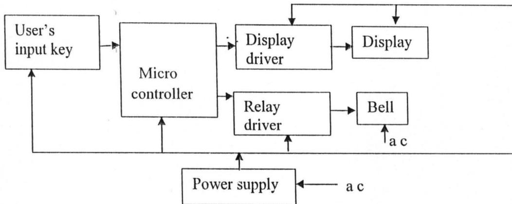
Fig 2.1 Block diagram of automatic College Bell
