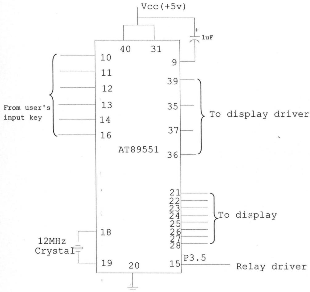
Fig 3.4 Circuit Diagram of Microcontroller Unit
