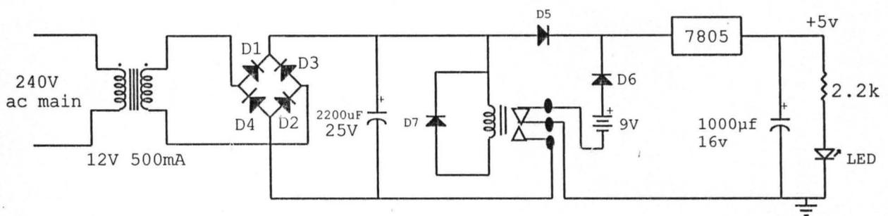
Fig 3.2 Circuit Diagram of Power Supply Unit
