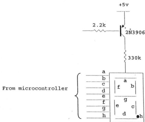
Fig 3.5 Circuit Diagram of Common Anode Display
