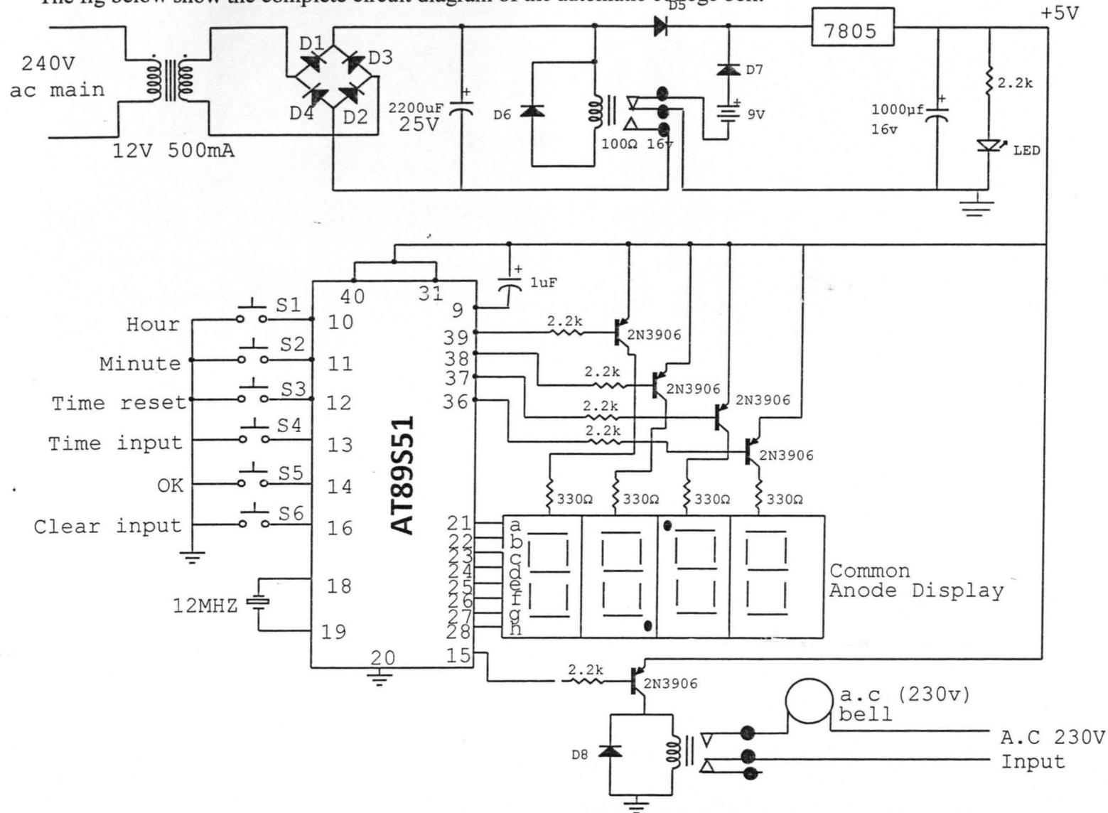
Fig 3.8 Circuit Diagram of Automatic College Bell
