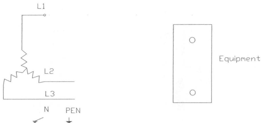
**Fig 4.2: A TN-C Earthing system (Combined Neutral and Earth throughout)**
