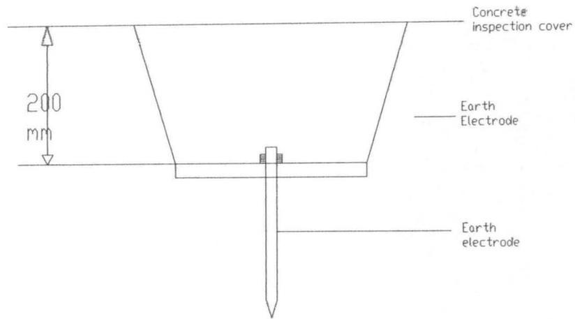
**Fig 4.4: Earth Electrode installation**
