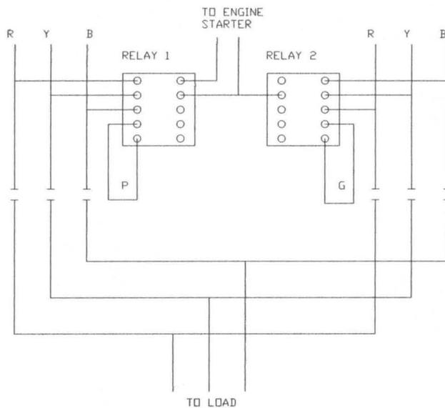
**Fig 3.2: Automatic equipment transfer switching**
