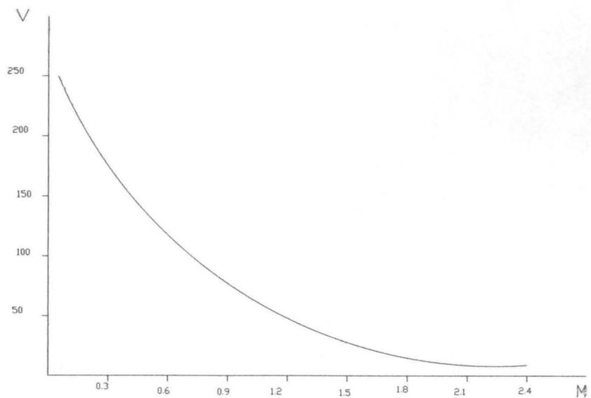
**Fig 4.5: Voltage distribution at surface of the ground due to the rod electrode**
