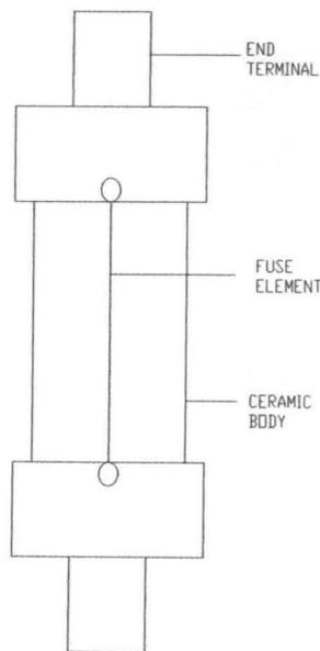
**Figure 4.1: A typical cartridge fuse**
