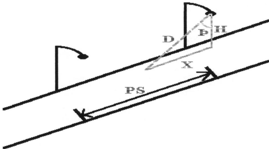
Fig 3.2: Pole spacing
