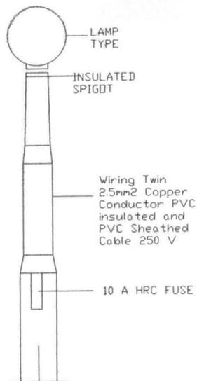
**Fig 3.1.1: A Typical top-post luminaire**
