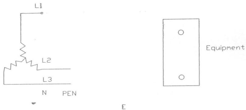
**Fig 4.3: A TN-S Earthing system (Combined Neutral and Earth separated)**
