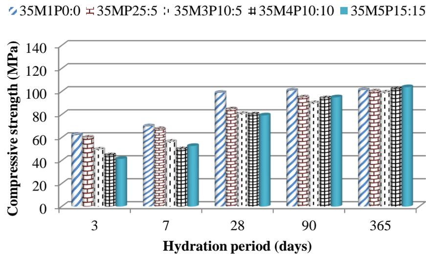
**Fig. 2** Compressive strength development of various SCCM (W/B = 0.35)
