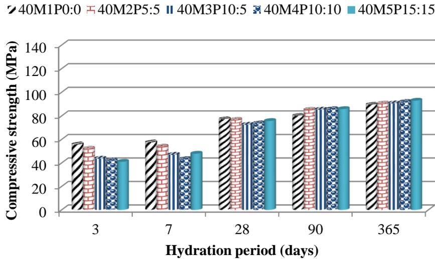
**Fig. 3** Compressive strength development of various SCCM (W/B = 0.40)
