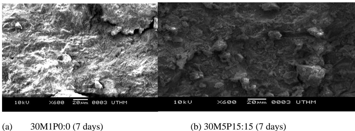
**Fig. 5** Microstructure of 0% and 30% blended SCHPC at 7 days
