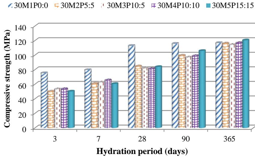
**Fig. 1** Compressive strength development of various SCCM (W/B = 0.30)
