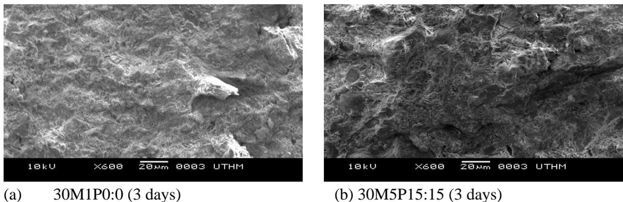
**Fig. 4** Microstructure of 0% and 30% blended SCHPC at 3 days
