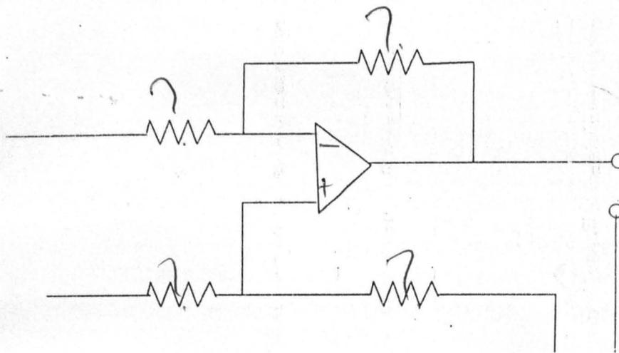
Voltage Difference Amplifier Circuit Diagram
