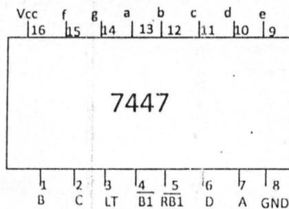
FIG 3.8 Pin Configuration of a 7447
