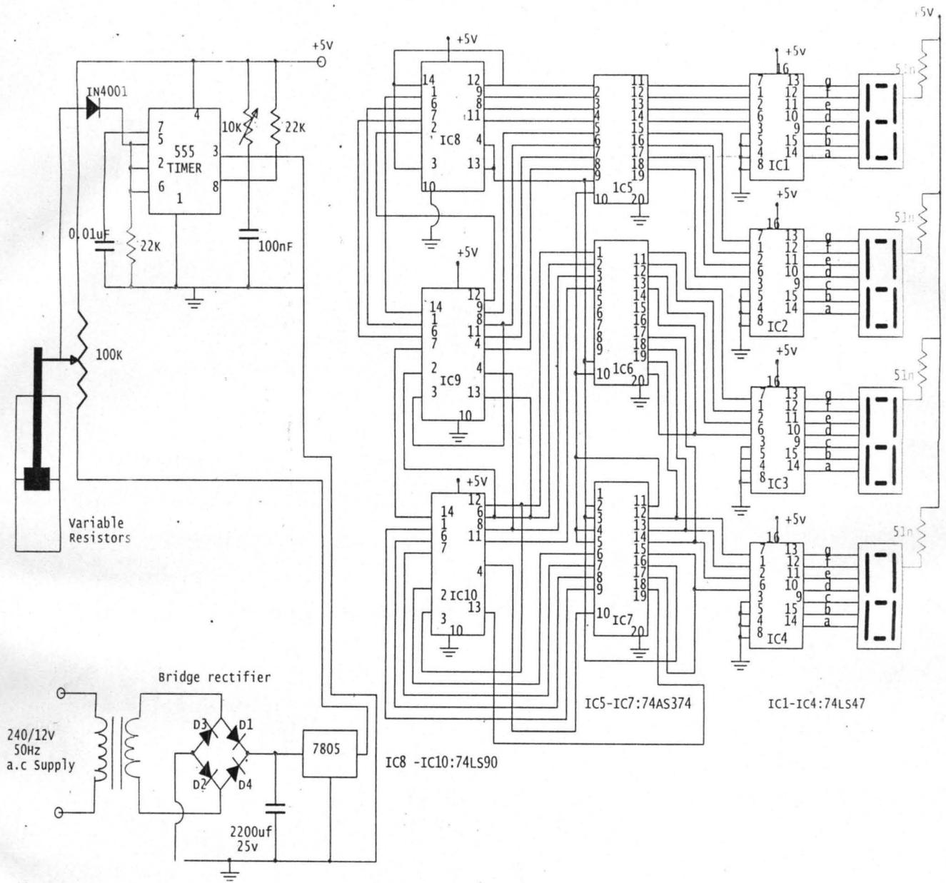
Circuit Diagram of a water leakage detector
