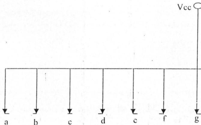
Common Anode Seven Segments Display Configuration.
