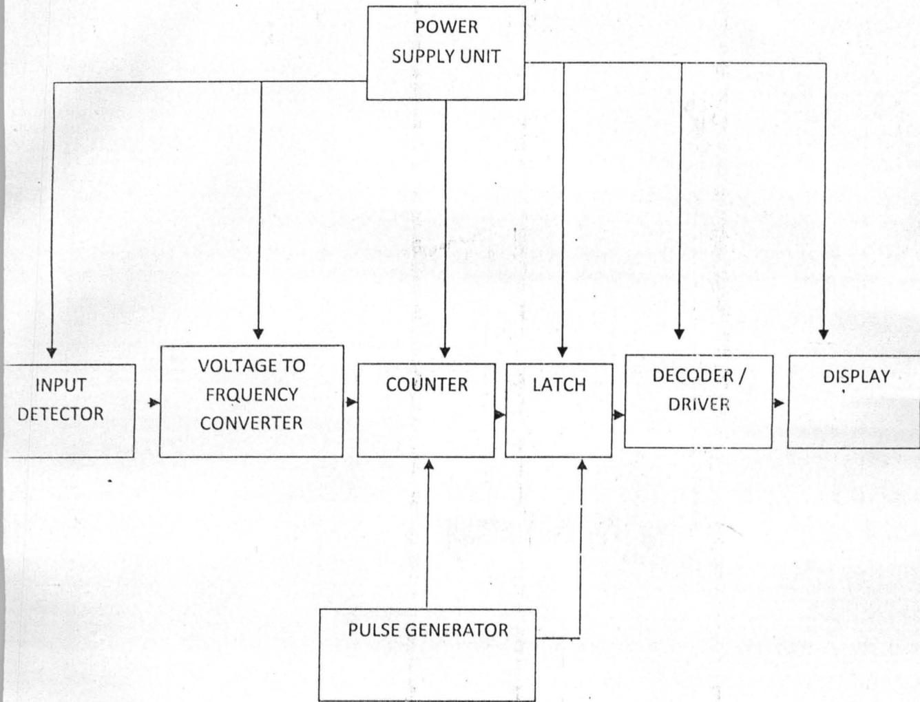
FIG1.1 BLOCK DIAGRAM OF A WATER LEAKAGE DETECTOR
