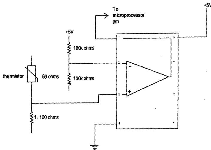
Fig 3.3 Circuit Diagram Of The Temperature Sensor
