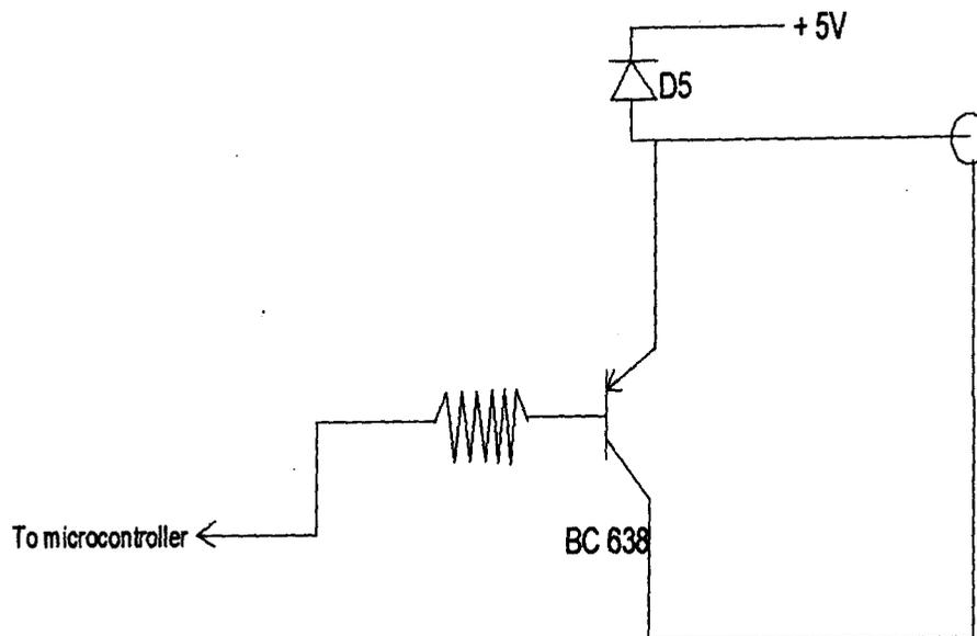
Fig 3.6 Transistor Switching Circuit For Select And Scroll Button
