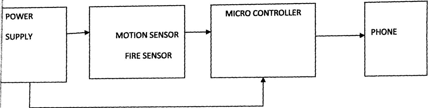
Fig 3.1 Block Diagram of the Home Security System
