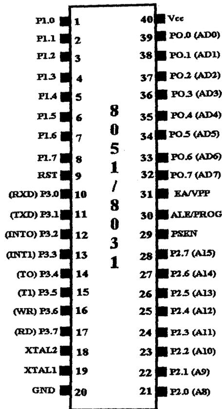
Fig 3.7 Pin diagram of the 8051 Microcontroller
