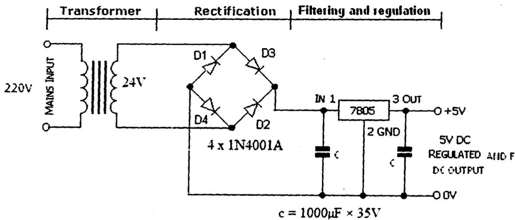
Fig. 3.2 Circuit Diagram Of Power Supply Unit
