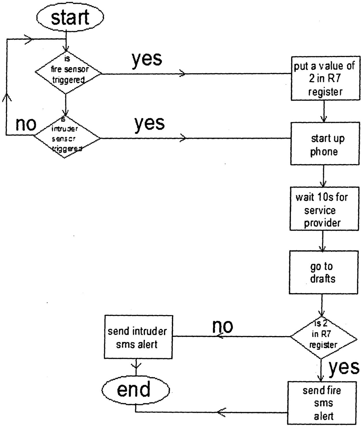
Fig 3.8 Microcontroller Flowchart
