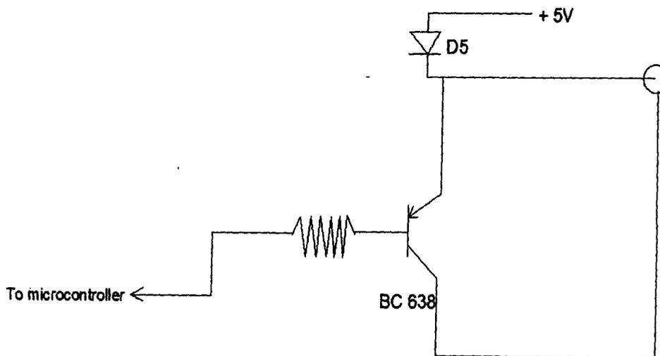
Fig 3.5 Transistor Switching Circuit For The Power Button
