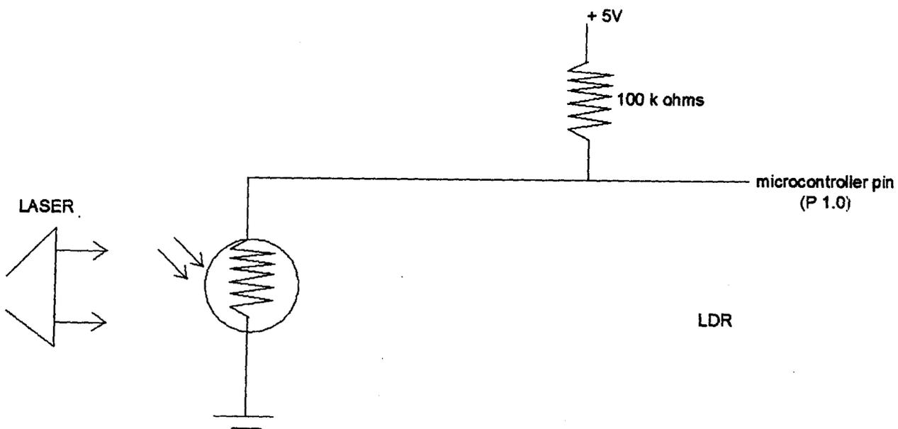
Fig 3.4 Circuit Diagram Of The Motion Sensor
