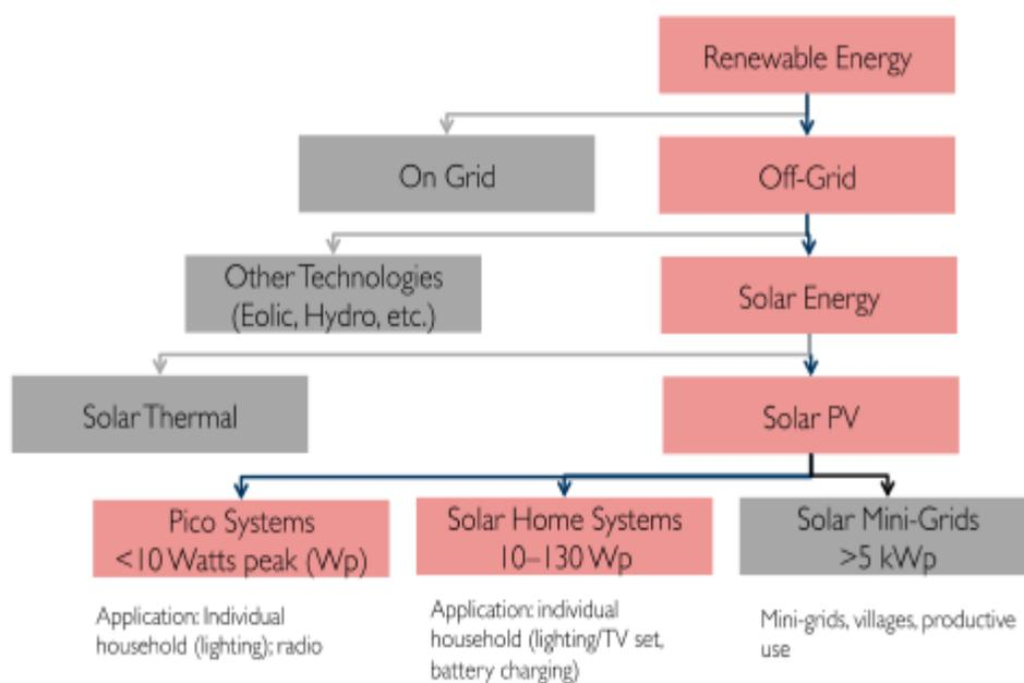
**Figure 2.3: Types of solar PV system**
