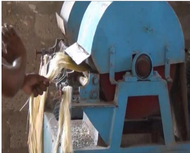
**Plate I11:** Banana Fiber Extracting Machine (Rahamaththulla*et al.*, 2018).
