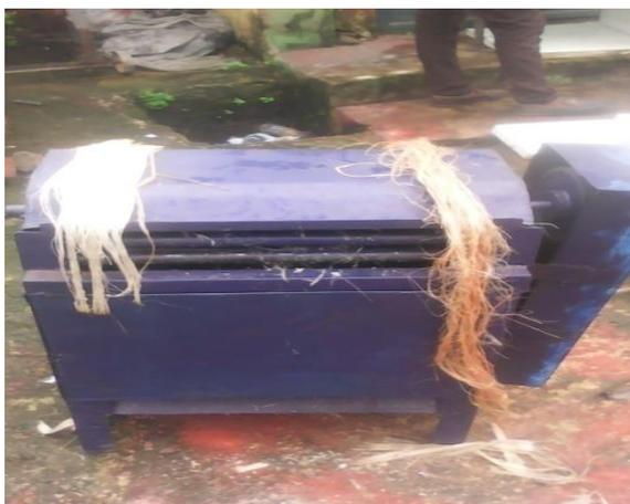
**Plate X:** front view of designed banana fiber machine
