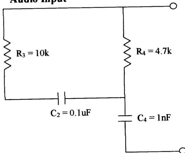
**Fig 3.2: Circuit diagram of audio coupling network**
