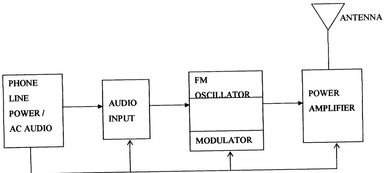
**Fig 3.1: Block diagram of Telephone bug FM Transmitter**
