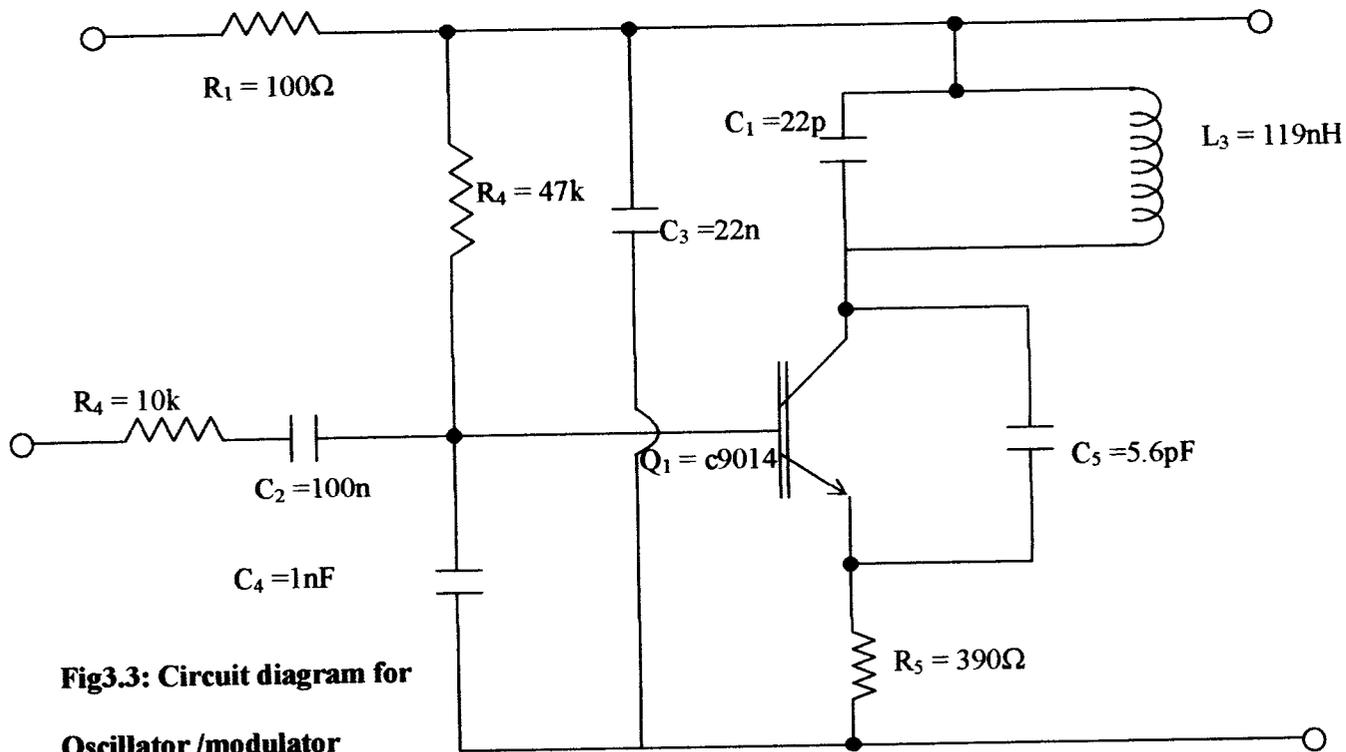
**Fig3.3: Circuit diagram for Oscillator /modulator**
