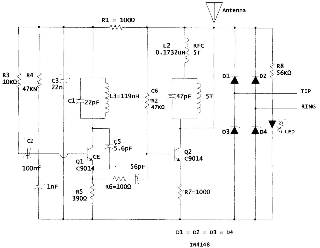
**Fig 3.12: The overall circuit diagram**
