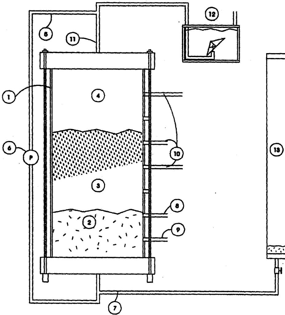
Figure 2.3: Laboratory Batch Reactors
