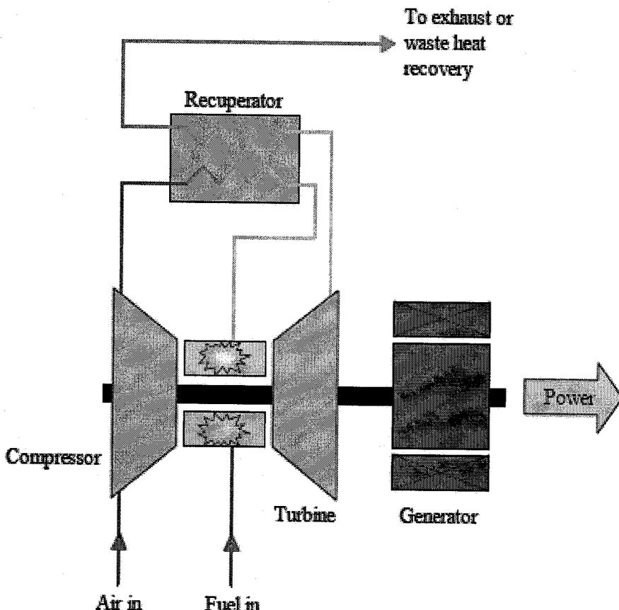
Figure 2.6: Operating Principle of a Gas Turbine
