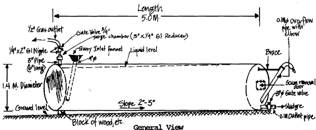
Figure 2.5: Plug Flow Digester
