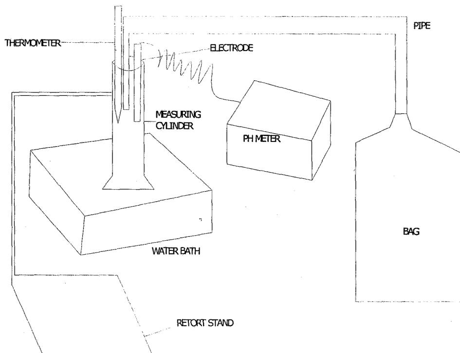
Figure 3.1: Experimental Set up for the Production of Biogas
