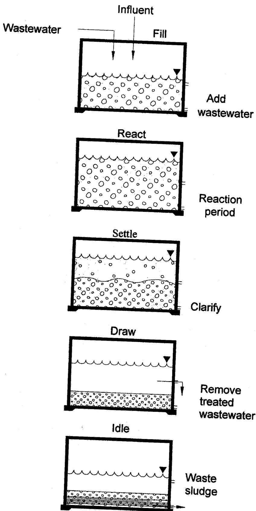
Figure 2.2: Operation of the Anaerobic Sequence of a Batch Reactor
