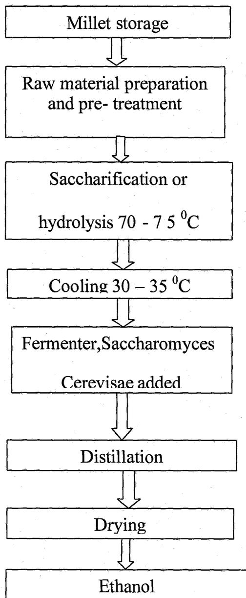
**Figure 2.1: Block Diagram for Ethanol Production from Millet**
