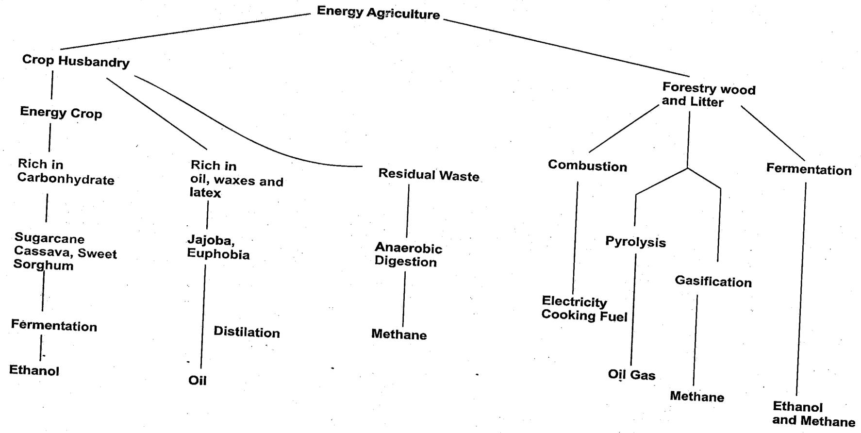
**Fig.2 Energy Agriculture: the Processes through which bio fuel can be obtained (Voce, and Blixt, 1984)**
