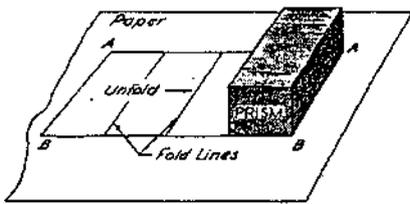
Figure 2.1 Development of a prism
