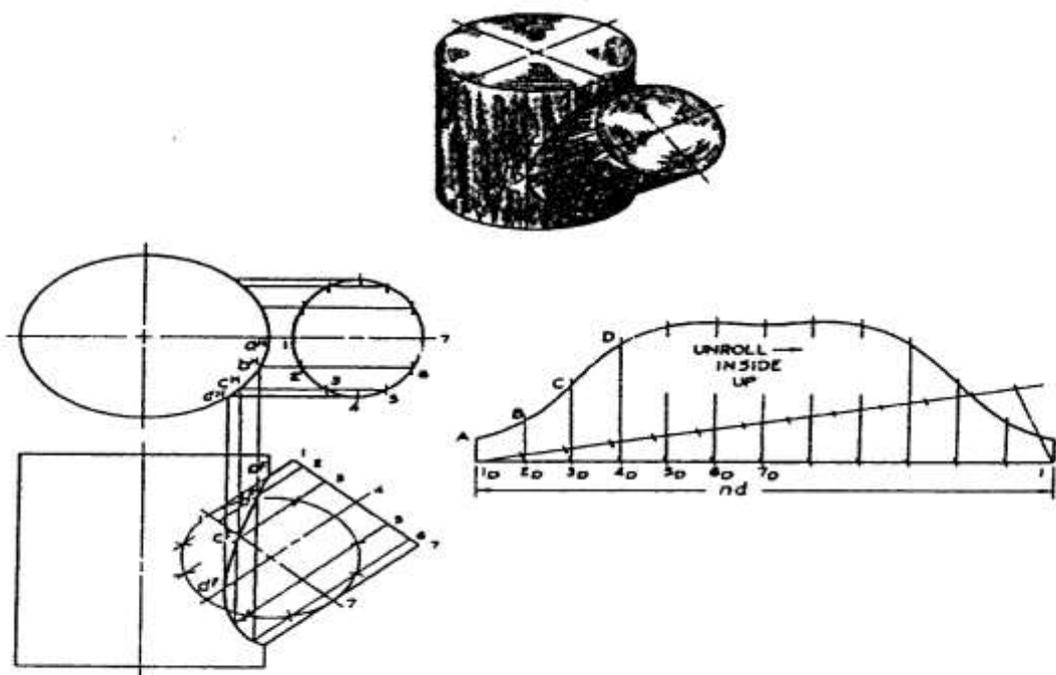
Figure 2.37 Intersecting cylinders
