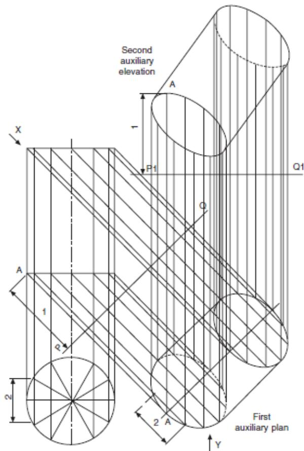
Figure 7 Auxiliary projections from a cylinder
