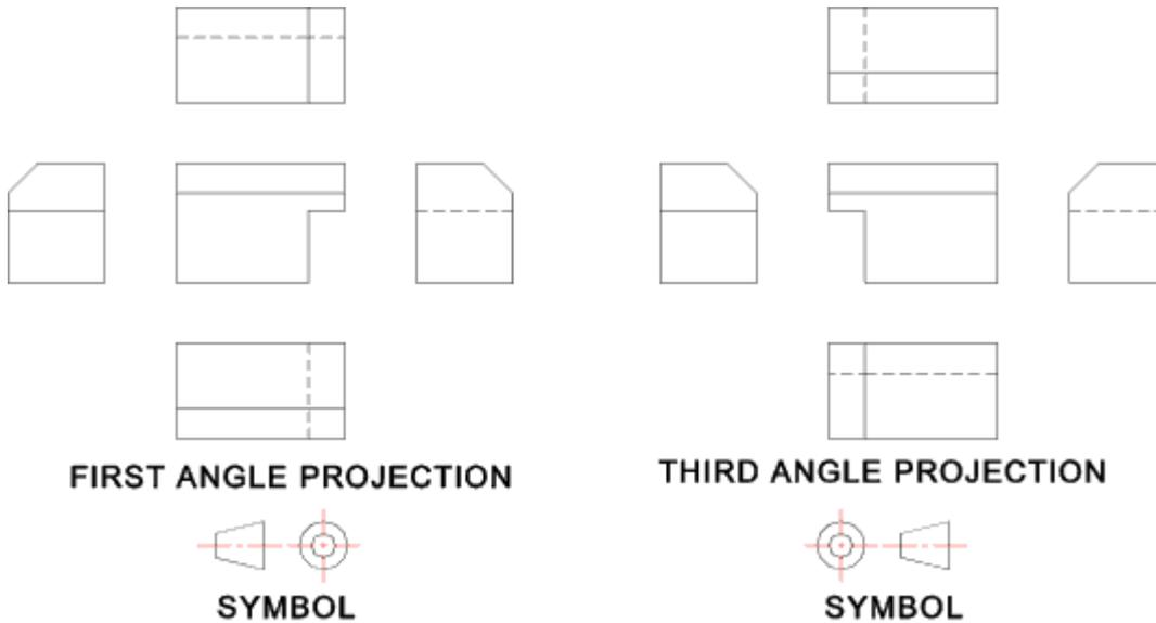
The symbol identifying the type of projection used should be placed in a space provided in the drawing block
