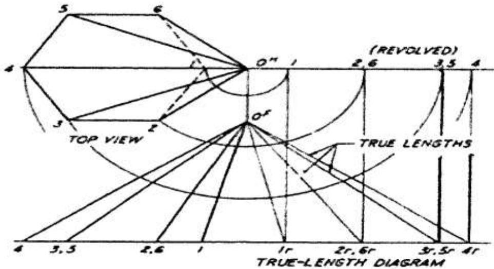
Figure 2.11 Development of a rectangular right pyramid
