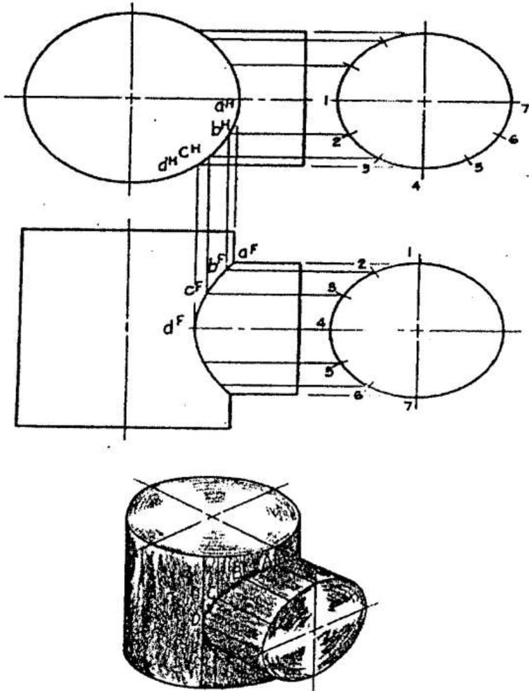
Figure 2.36 Intersecting cylinders
