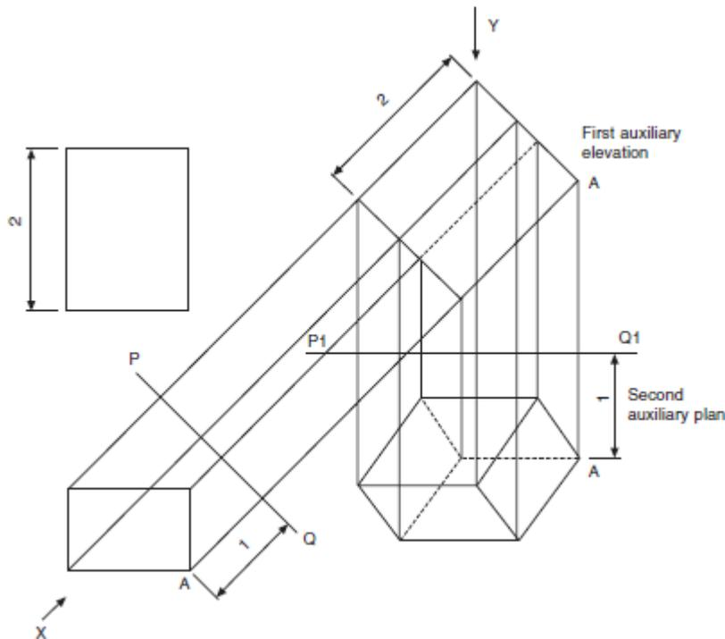
Figure 3.5 Isometric projection of a rectangular box from end view
