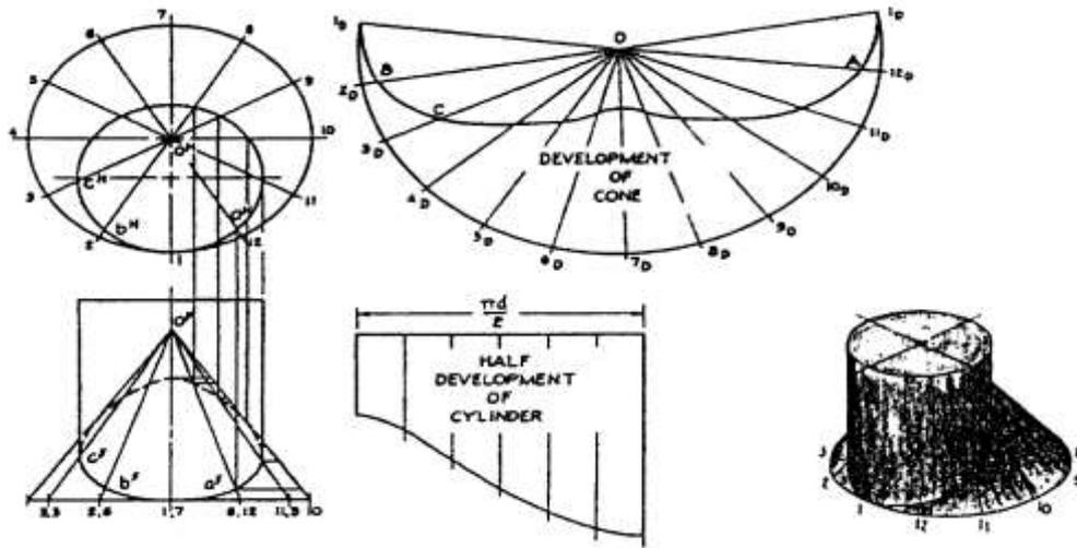
Figure 1.39 Intersecting cylinder and cone
