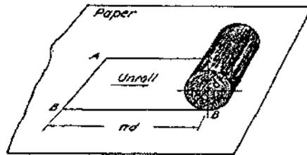
Figure 2.3 Development of a cylinder
