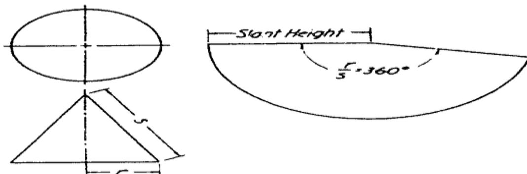
Figure 2.13 Development of a right cone
