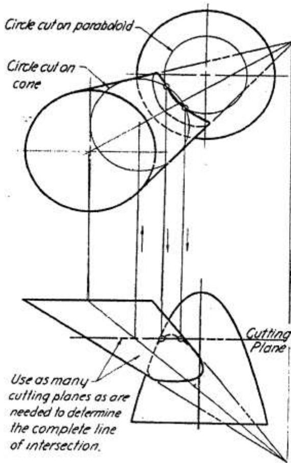
Figure 1.42 Intersecting cone and paraboloid
