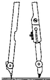
(a) Sharpening and position of compass lead
