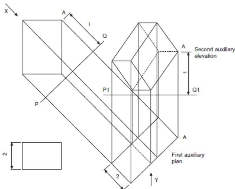
Figure 3.4 Isometric projection of a rectangular box from plan view
