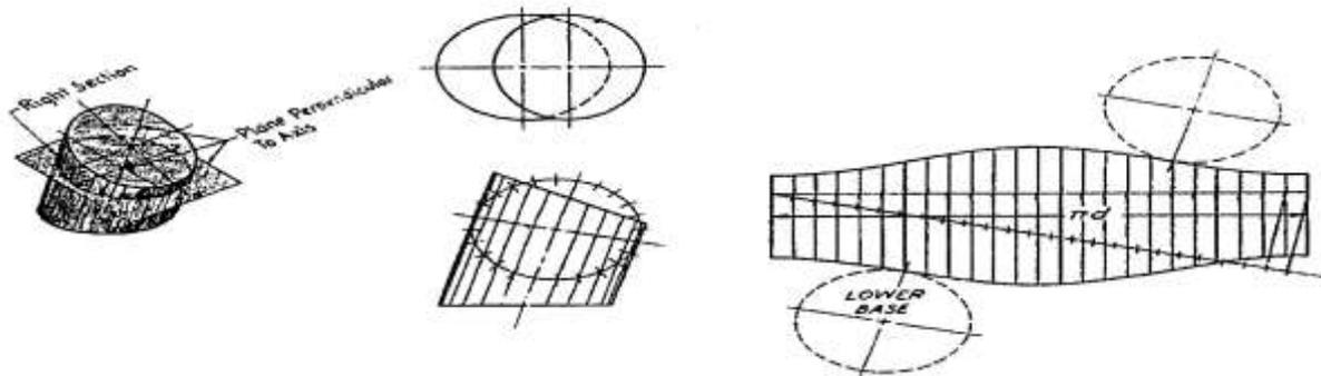
Figure 2.9 Development of an oblique cylinder
