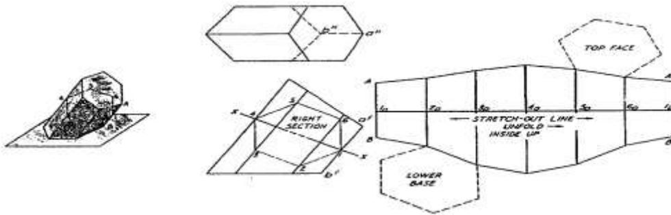
Figure 2.6 Development of an oblique prism
