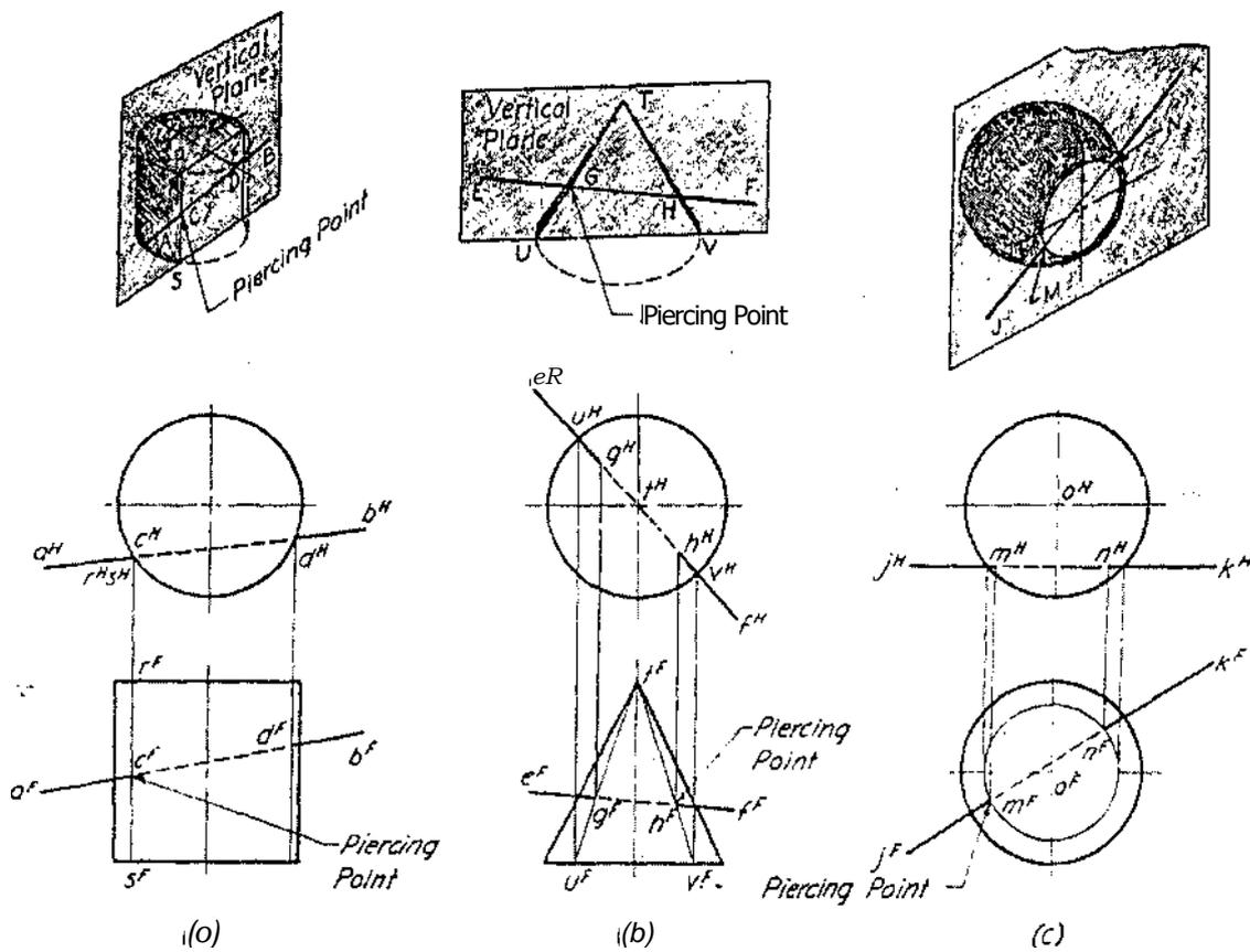
Figure 2.25 Use of line projection-plane
