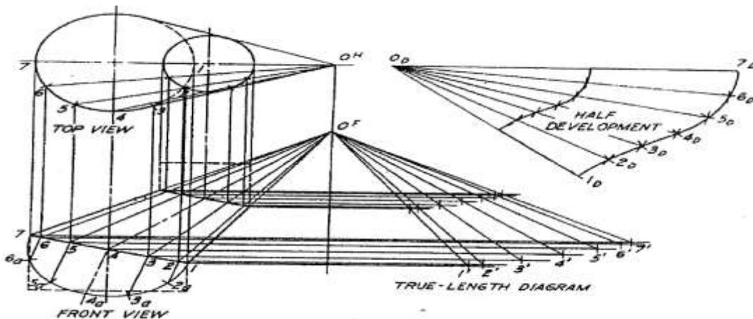
Figure 2.20 Transition piece connecting two pipes
