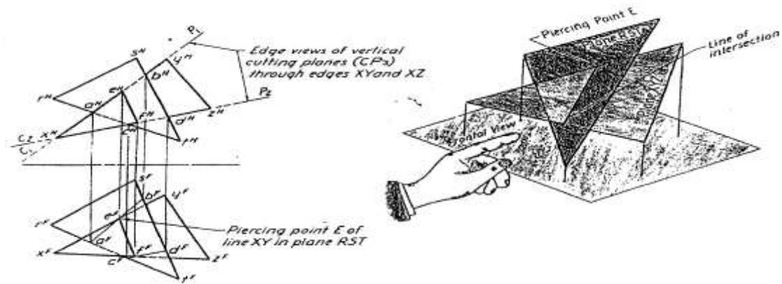
Figure 2.28 To find the intersection line of two planes
