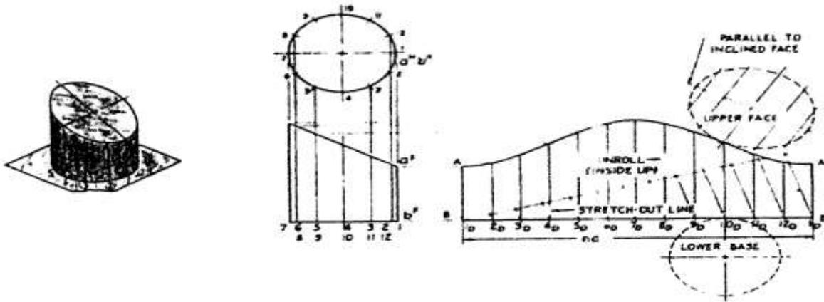
Figure 2.7 Development of a right circular cylinder
