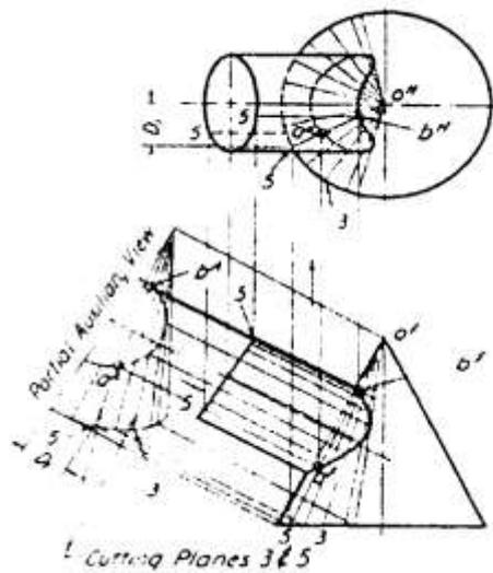
Figure 2.40 To find the intersection of a cone and a cylinder
