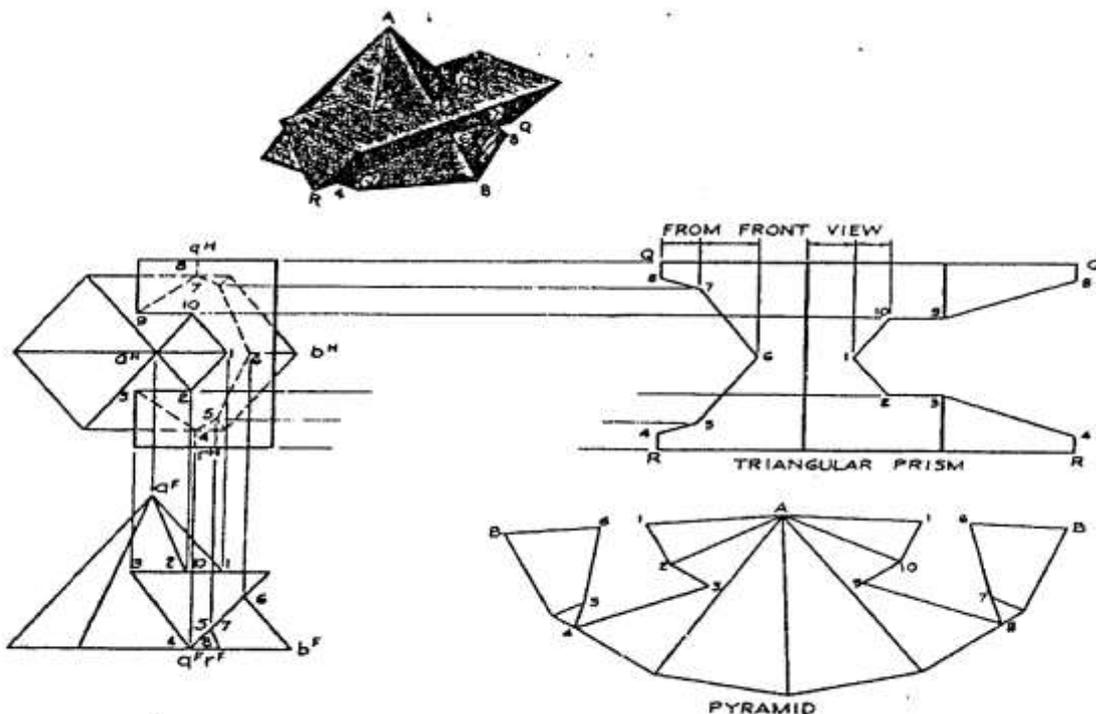
Figure 2.34 Intersecting pyramid and prism
