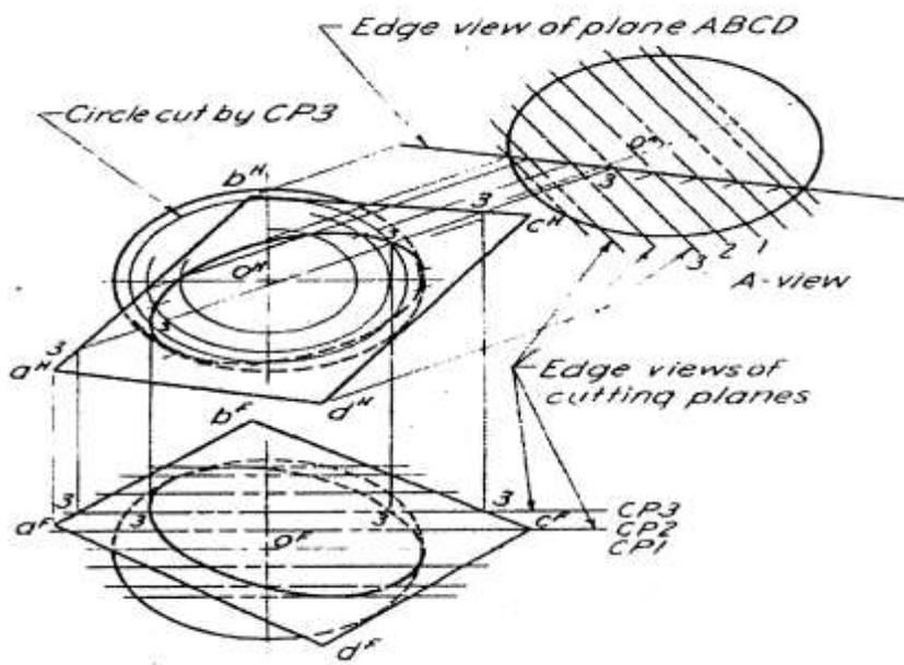
Figure 2.31 To find the intersection of a sphere and an oblique plane
