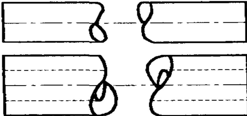
**Fig. c** Break lines for circular parts, solid or hollow
