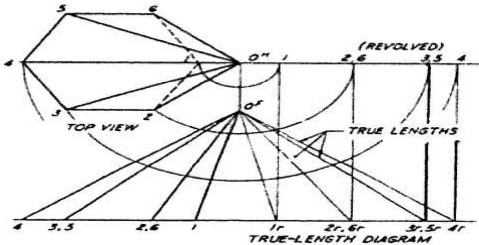
Figure 2.10. True-length diagram (the revolution method)
