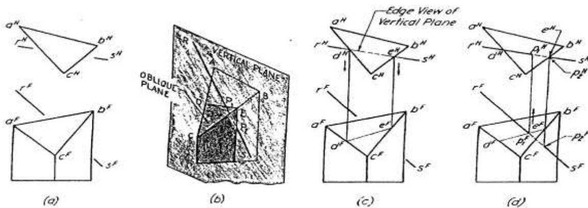
Figure 2.25 Use of a line-projecting plane
