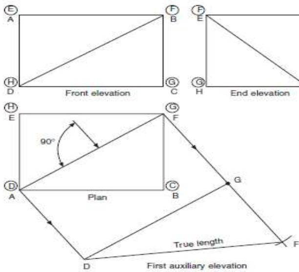
Figure 3.2 Projection of true length of line
