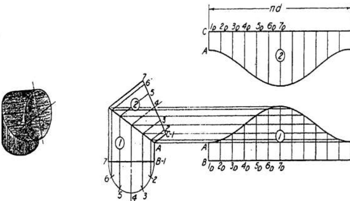
Figure 2.8 Two-piece elbow
