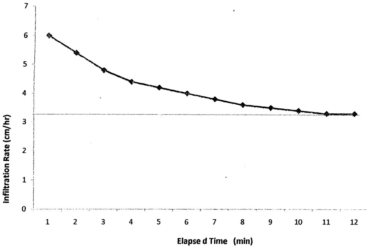
**Fig. 4.14: Infiltration rate of soil in the middle part of gully area (CH 0 + 490)**
