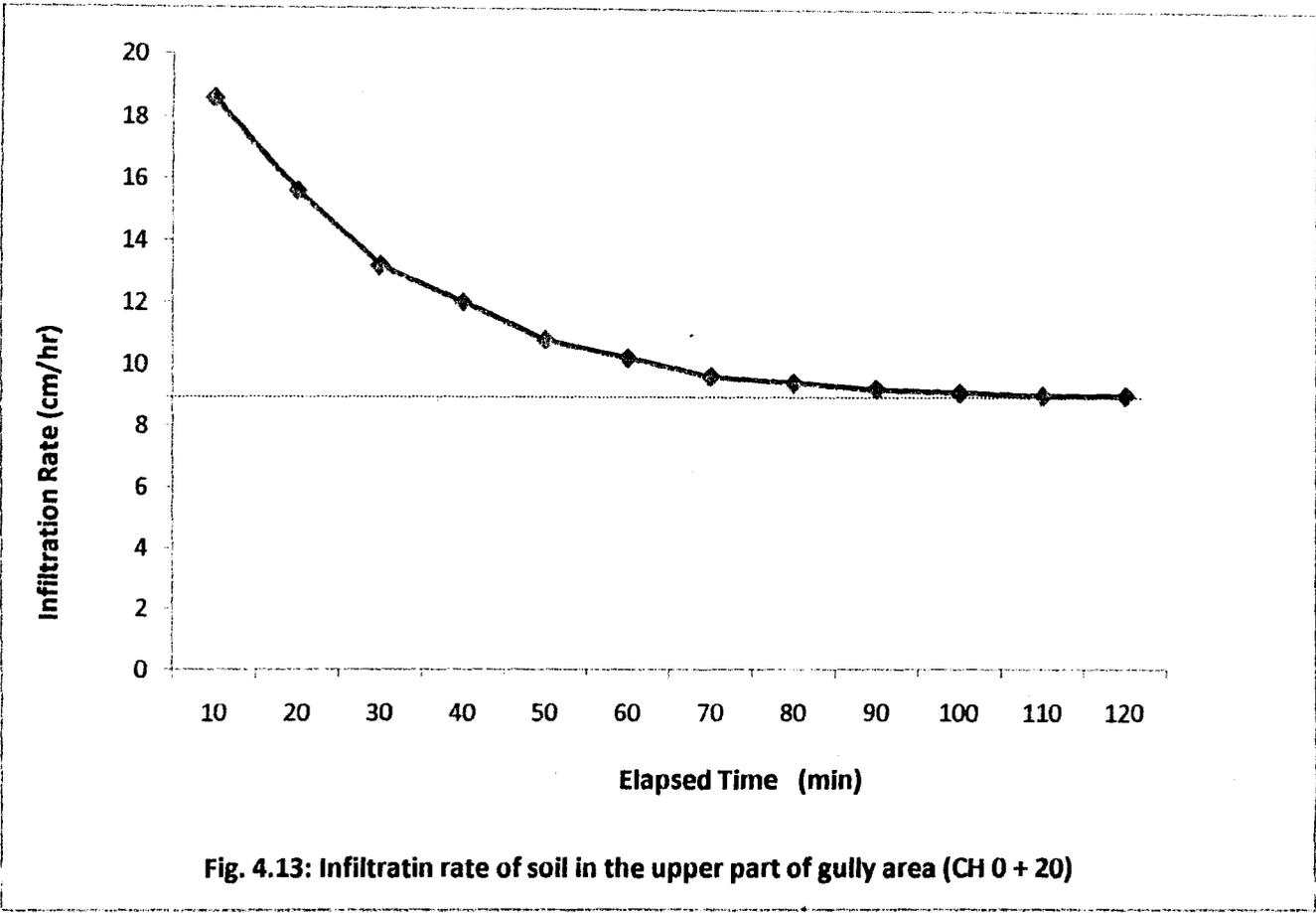
**Fig. 4.13: Infiltratin rate of soil in the upper part of gully area (CH 0 + 20)**
