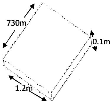
Fig 4.21: Volume of concrete required for blinding
