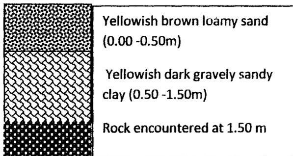
**Fig 4.5: Soil profile loggings of naturally occurring soil layers in the project site**
