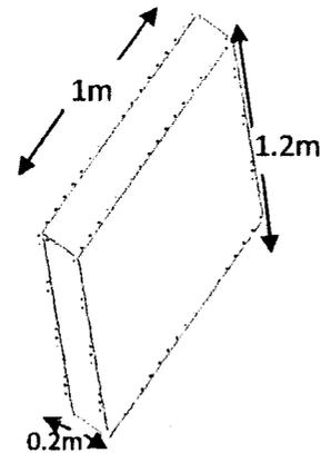
Fig 4.22: Volume of concrete required per metre length of wall
