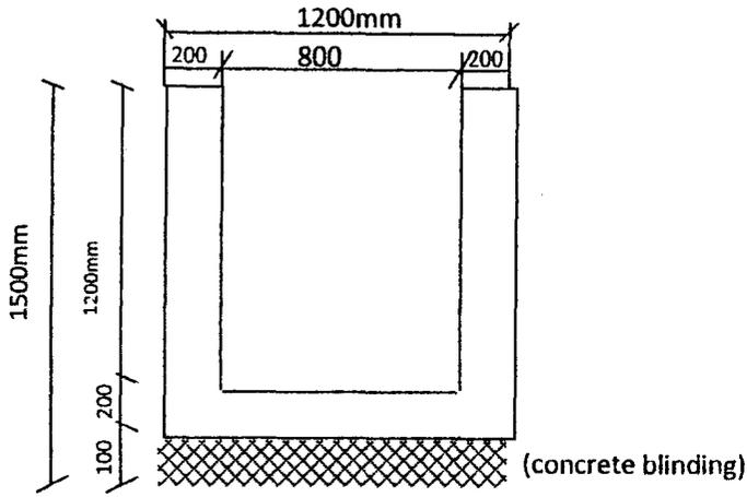
Fig. 4.17: Typical designed drain section
