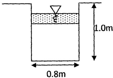
Fig. 3.2: Designed drainage channel
