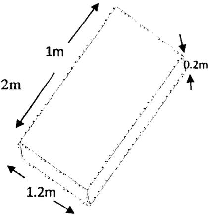
Volume of concrete per metre length of walls and base =  $0.48 + 0.24$
