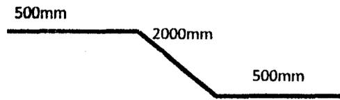
**Fig. 4.29: Shape and dimension of bar for drop structure**
