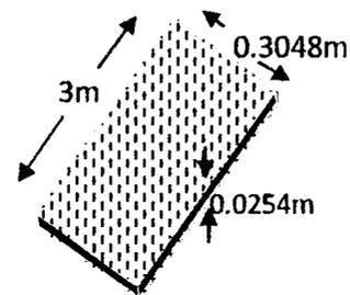
Fig 4.20: Size of wood for formwork
