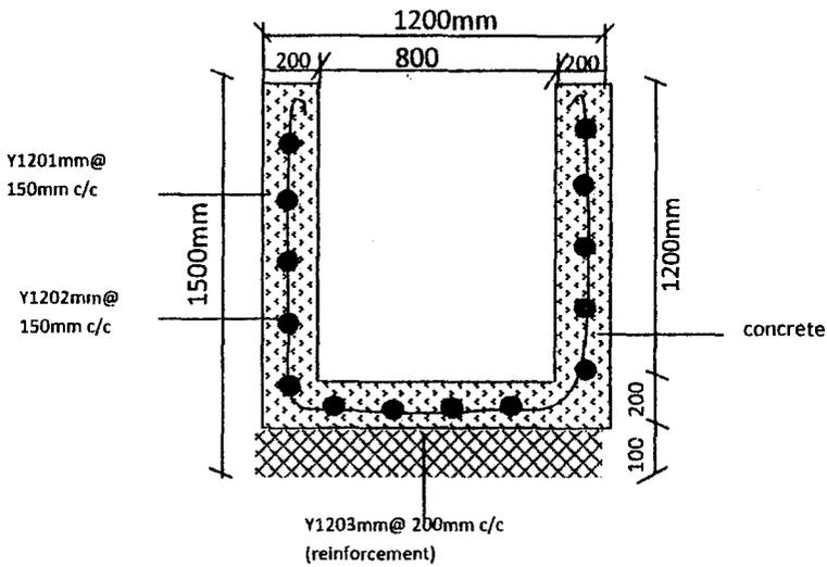
Fig.4.18: Typical designed drain section with reinforced concrete
