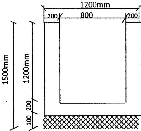
Fig. 4.24: Typical drain section
