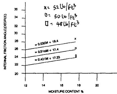
Fig.1.6b Variation of internal angle of friction with moisture content and density [Stewart, 1960].
