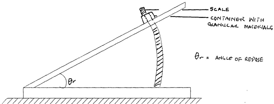
Fig 1.0 :Simple device for measuring angle of granular materials.
