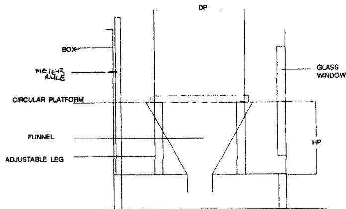
FIG. 2.4 DEVELOPED APPARATUS FOR MEASURING REPOSE ANGLE OF GRANULAR MATERIALS
