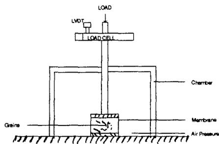
fig 1.5:Schematic for application of Triaxial compression test of agricultural grains.
