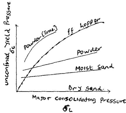
Fig.1.8: Critical flow factor FF of a hopper superimposed on flow function several solids (Jenike and Johnson Inc)
