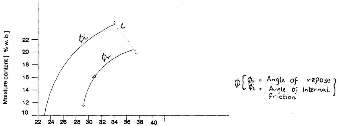
Fig 1.4:Variation of angle of repose and angle of internal friction with moisture content(Lorenzen, 1957).
