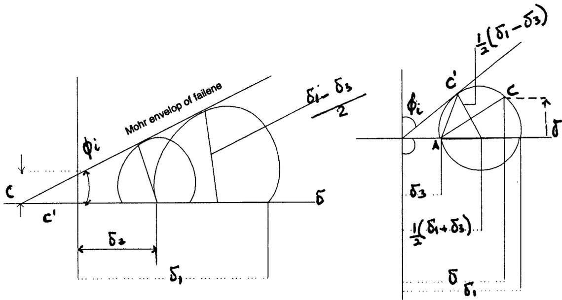
FIG. 1.3 : Mohr Circle And Mohr Envelope Of Failure
