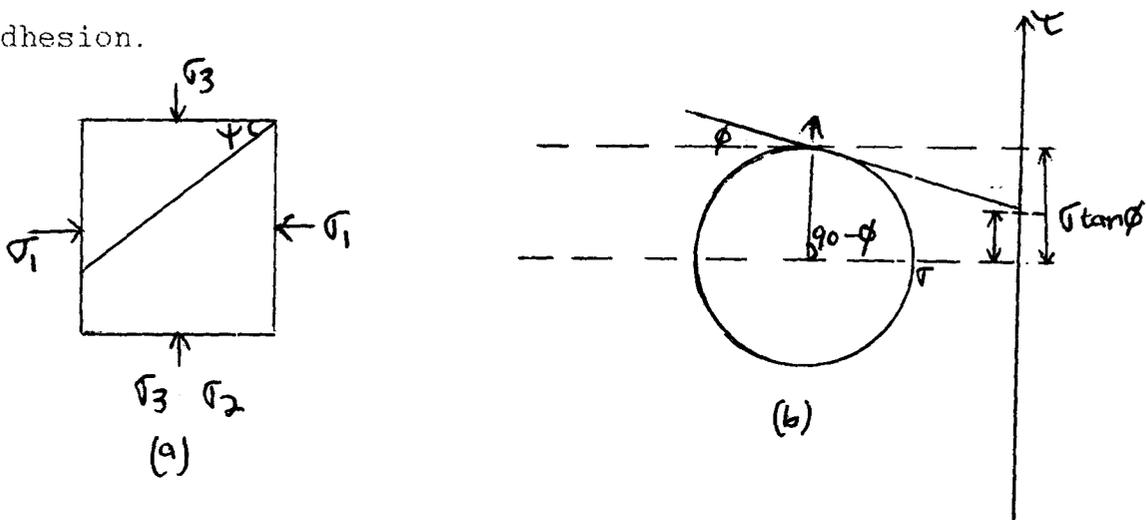
Fig. 1: Mohr-Coulomb Failure diagram
