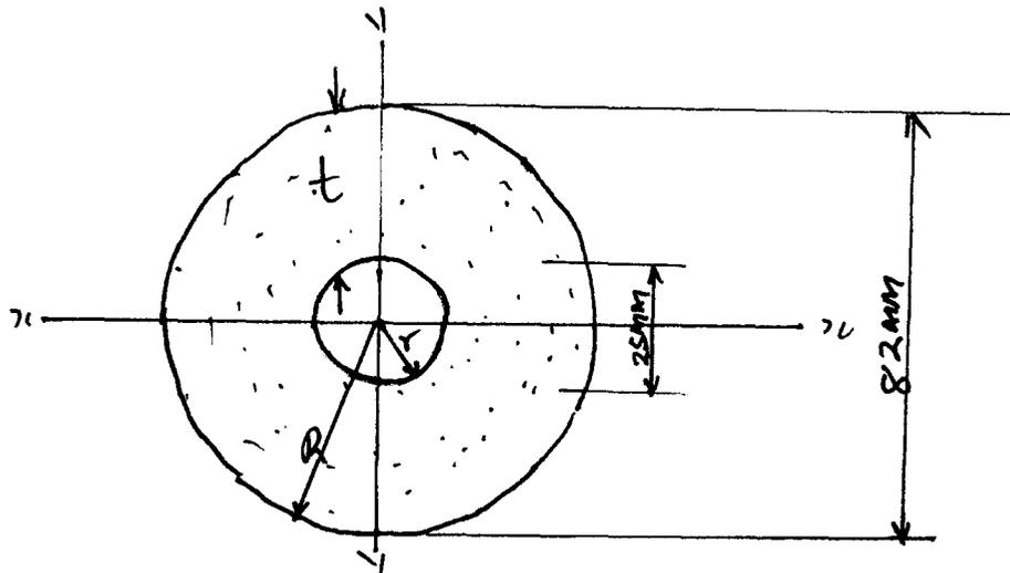
The metal use for the construction is gauge 12 which the thickness is assume to be 2.526mm. The metal is welded to the cylinder casing at the bearing housing to protect the shaft from rubbing against the wall of the housing.
