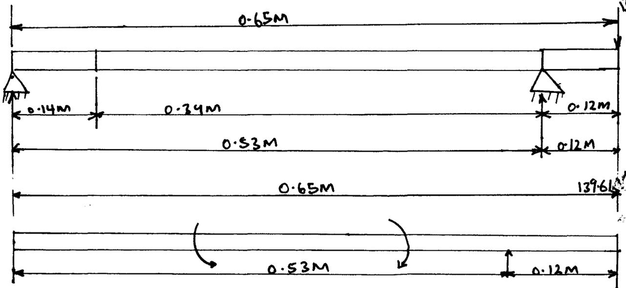
To determine the reaction  $R_A$  and  $R_C$  of the horizontal component.
