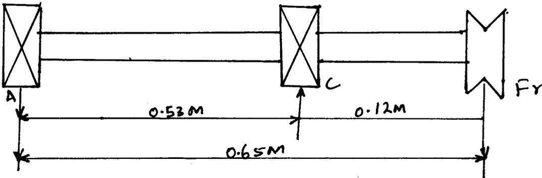
Fig I load on bearing
