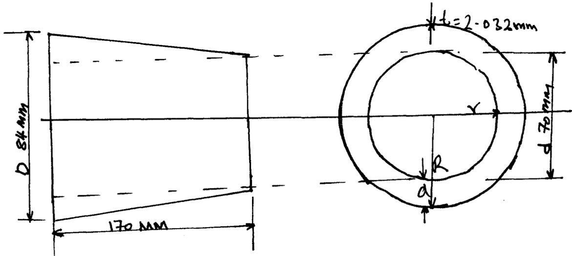
The use of gauge 16 metal mild sheet which has a thickness of 2.032m.
