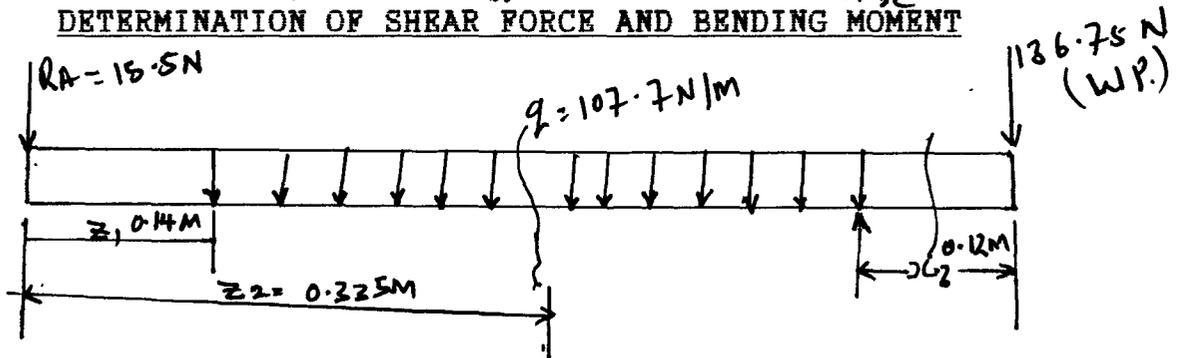
However, the shear force and bending moment can be determines as follows:-
