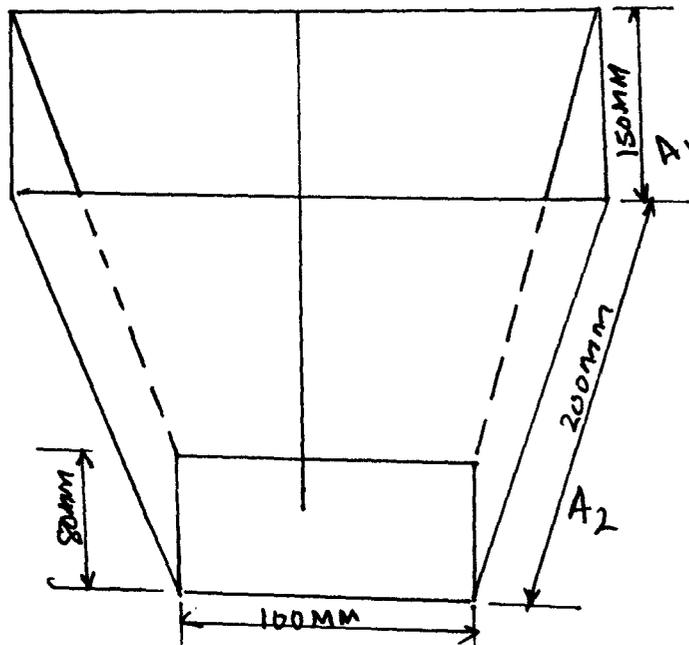
The hopper is constructed with carbon mild steel of gauge 18 which is 1.219mm.
