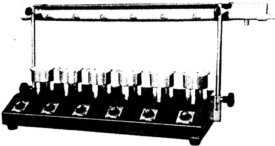
**Plate 3.5: Micro Kjeldahl Digestion Unit**
