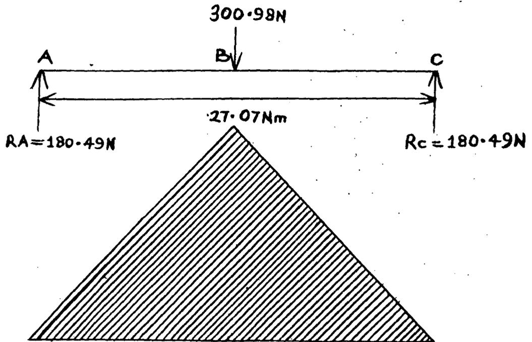
Fig.6: BENDING MOMENT DIAGRAM ACTING ON THE SHAFT.
