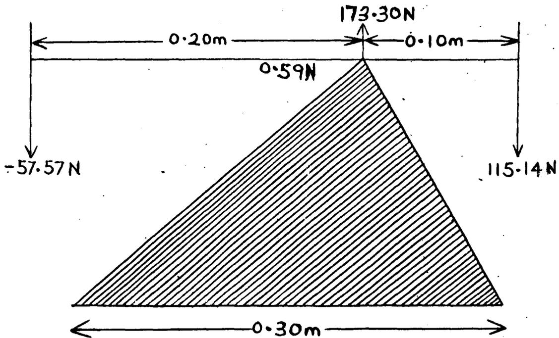
Fig.4 BENDING MOMENT DIAGRAM ACTING ON FRAME
