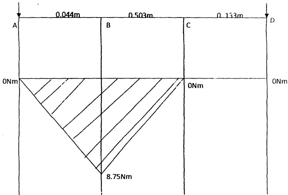
To calculate maximum bending load
