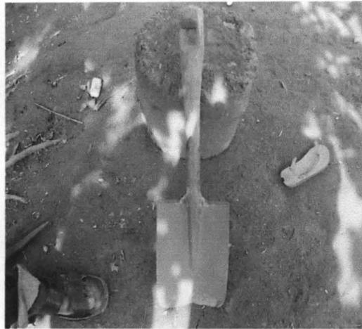
Plate III: Shovel used to pack the soil
