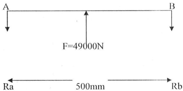
Fig 3.1 Shear force diagram
