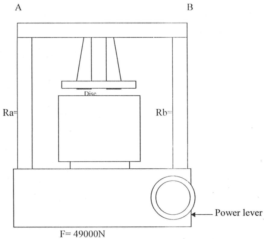
Fig. 3.0 Frame of Hydraulic press
