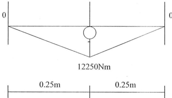
Fig. 3.2 Bending moment diagram
