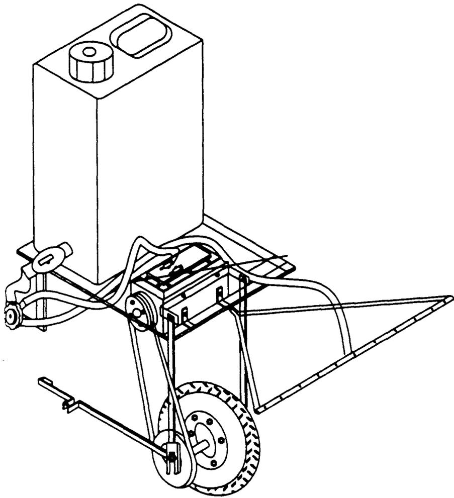
ISOMETRIC VIEW OF A MOTORCYCLE POWERED BOOM
