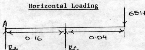
$$\begin{aligned} \sum M_A = 0: & -65(0.20) + 0.16R_C = 0 \\ & R_C = \frac{13}{0.16} = 81.3\text{N} \end{aligned}$$
