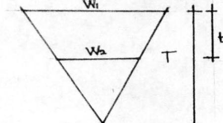
Fig. 3.4 Bottom width of V-belt
