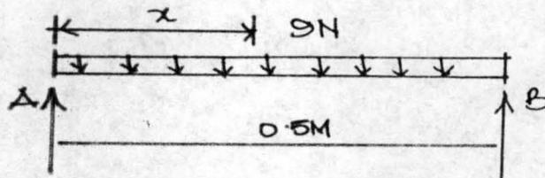
Fig 3-4. Showing the uniformly distributed load on AB
