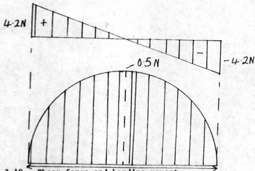
Fig. 3.10. Shear force and bending moment.
