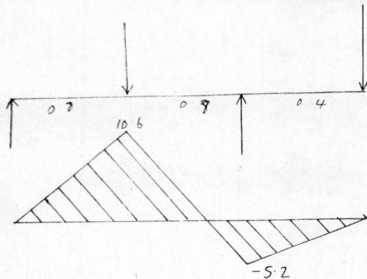
FIG 3-7-7 THE COMBINED BENDING MOMENT DIAGRAM
