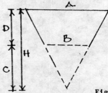
$$\begin{aligned}\text{Volume of small cone} &= \frac{1}{3} \pi r^2 x L \\ &= \frac{1}{3} \pi (0.1)^2 \times 0.03 \\ &= 0.00032\text{m}^3\end{aligned}$$
