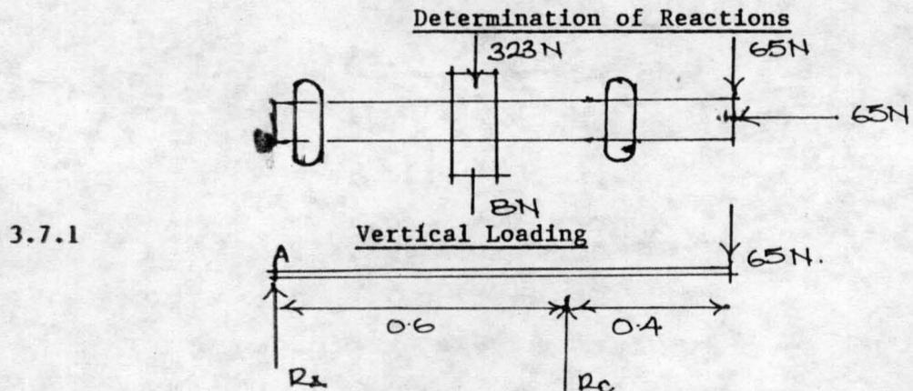
$$\begin{aligned} \sum M_A = 0: & -65(0.20) + (0.16)R_C - 330(0.08) = 6 \\ & -13 + 0.16R_C - 26.4 \\ & 0.16R_C = -26.4 + 13 \\ & R_C = \frac{39.4}{0.16} \end{aligned}$$
