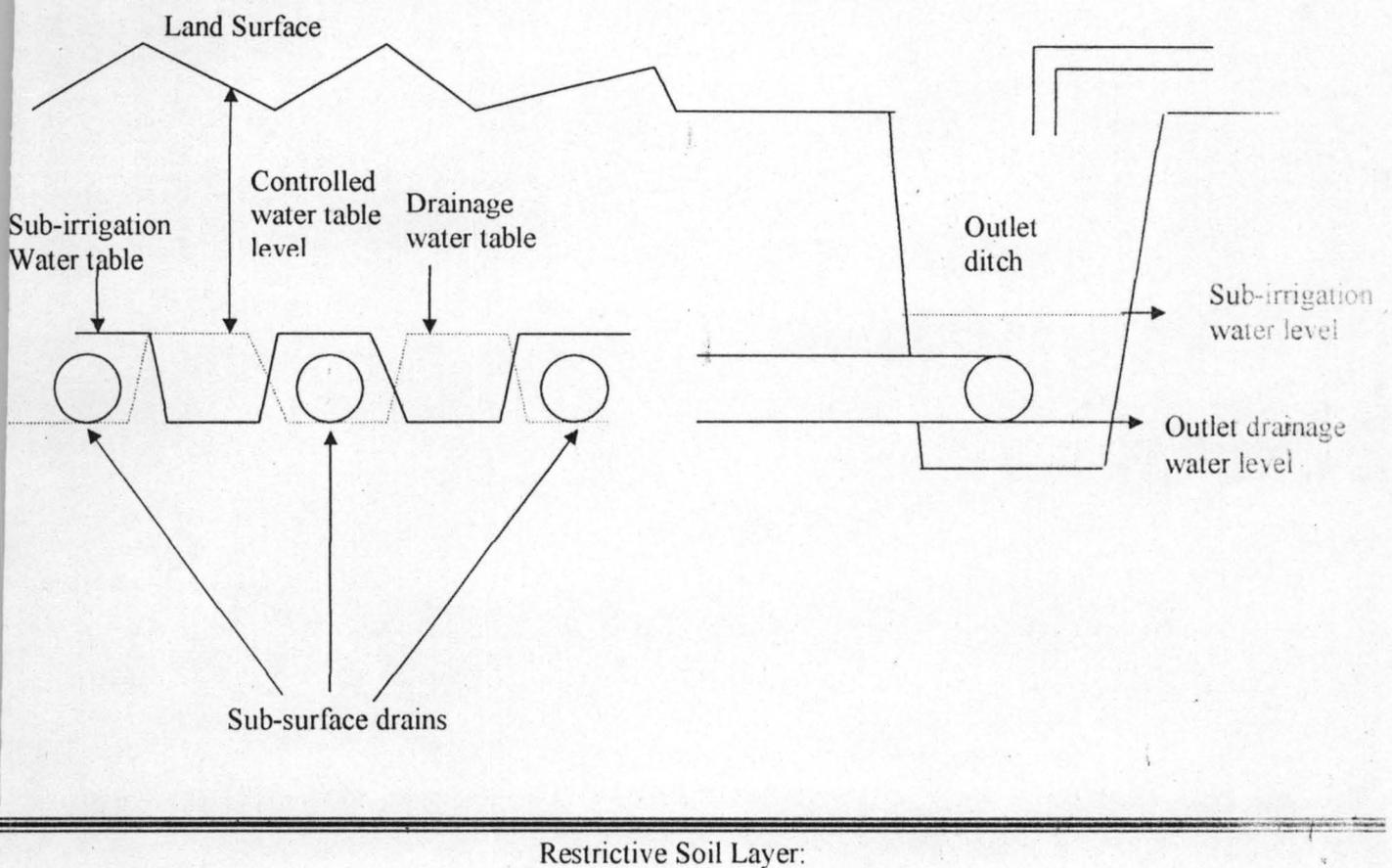
Fig 2.1 Water Table Control Structure
