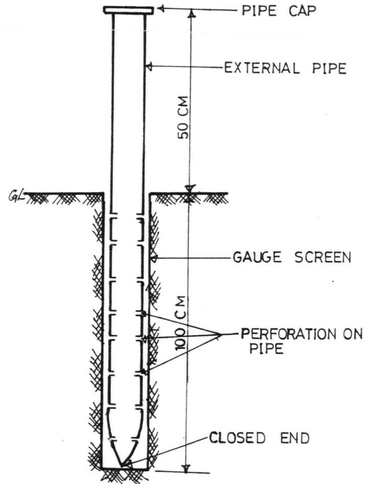
FIG 3:07 CROSS SECTION OF CONSTRUCTED PIEZOMETER PIPE
