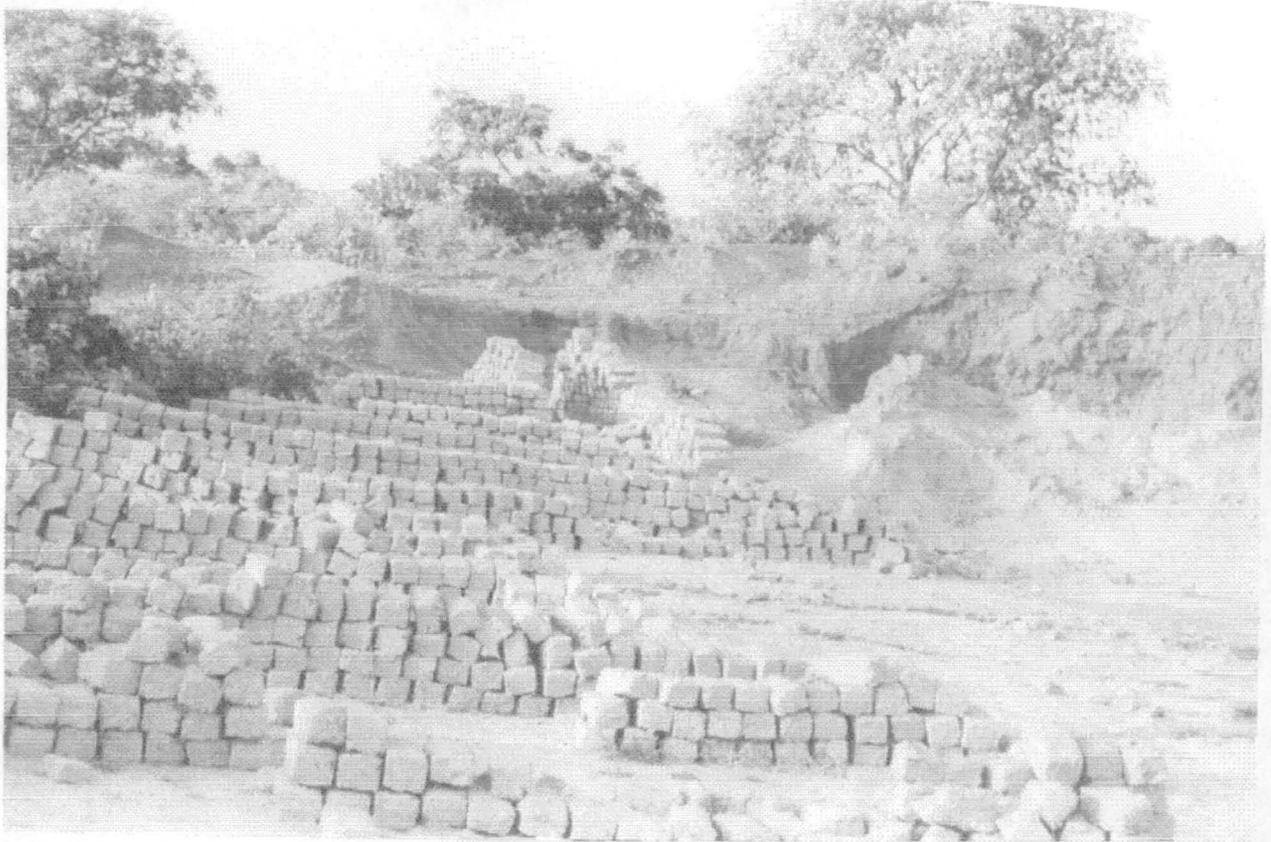
**Plate 7:- Showing bricks made from laterite at the bank of the reservoir.**
