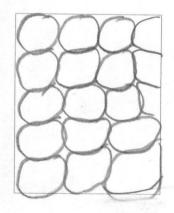
Spherical grains packed in such away that Voids or Pores make up appropriately 40% of the volume
