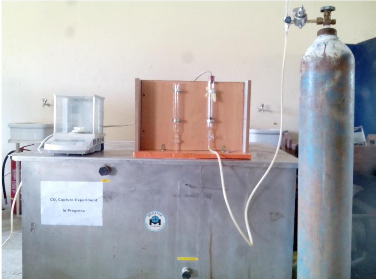
**Figure 3.3: Experimental setup for CO<sub>2</sub> Adsorption**
