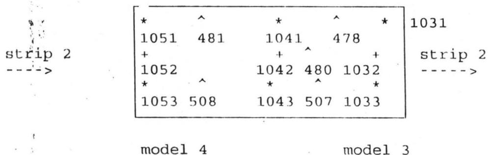
Fig 4 sketch showing models formed from photographs in strip two.
