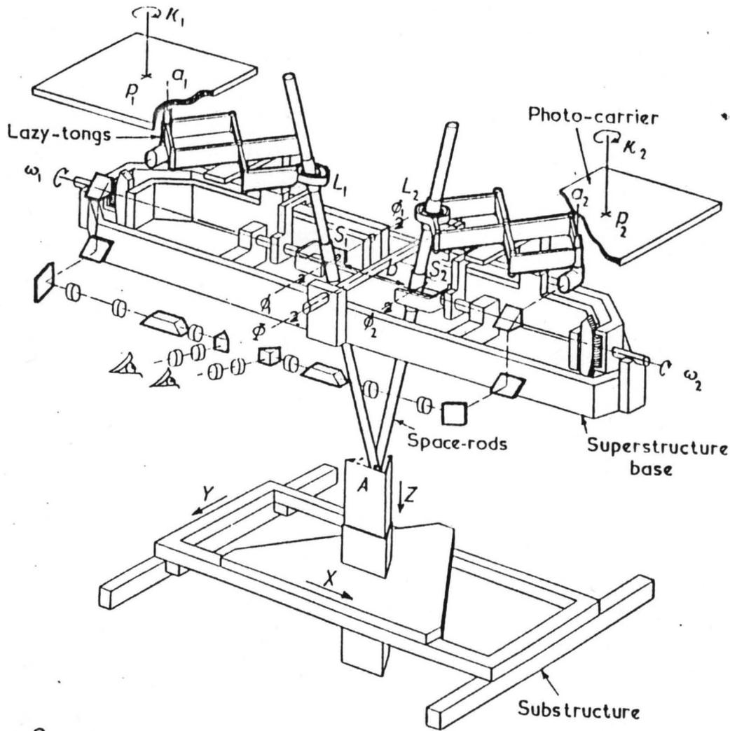
Fig 9. A8 autograph space-rod diagram. (Wild, Heerbrugg Ltd of Switzerland).
