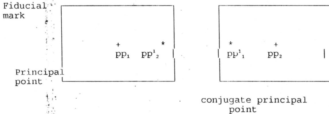
Fig 5 shows relative points of fiducial and principal point on adjacent photographs
