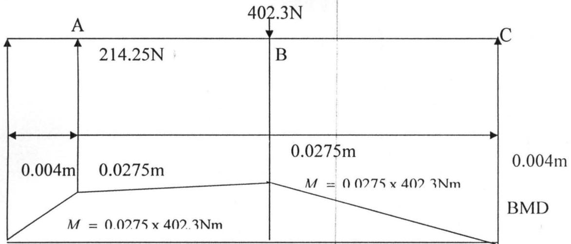
**Fig. 5:** Bending Moment at Horizontal Loading
