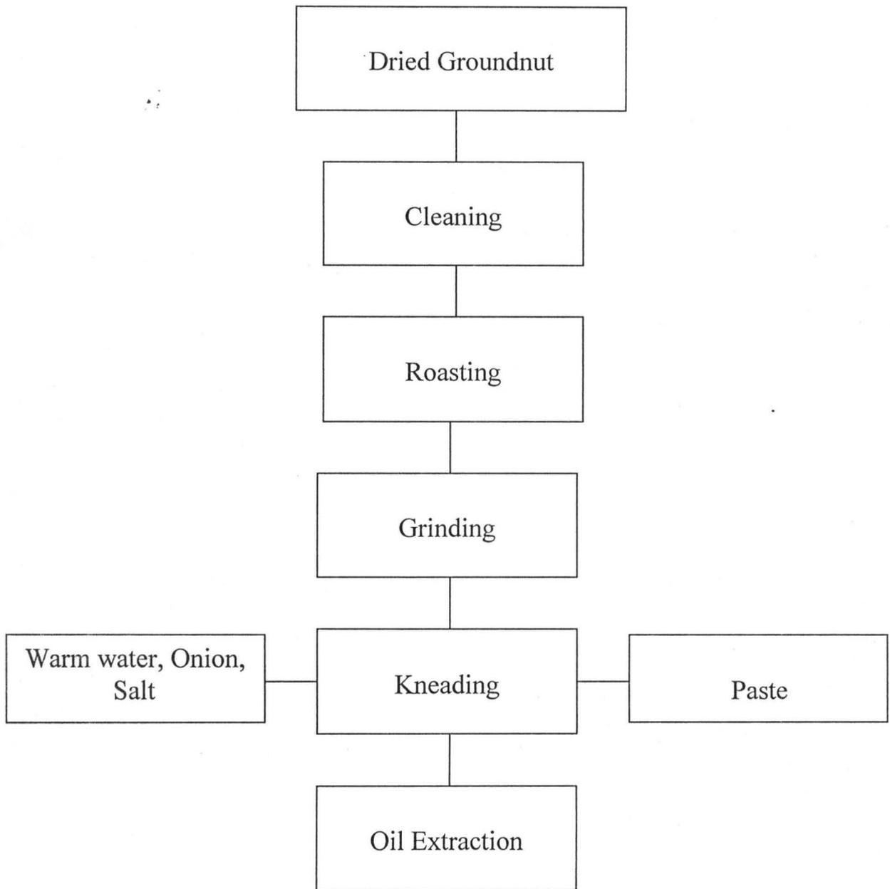
**Figure 1: Flow Chart of Groundnut Processing for Oil Extraction**
