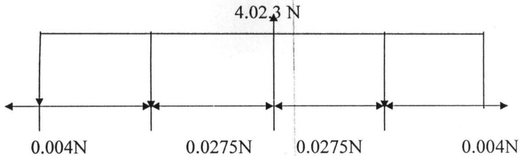
**Fig. 4: Free Body Diagram of Press Bar**
