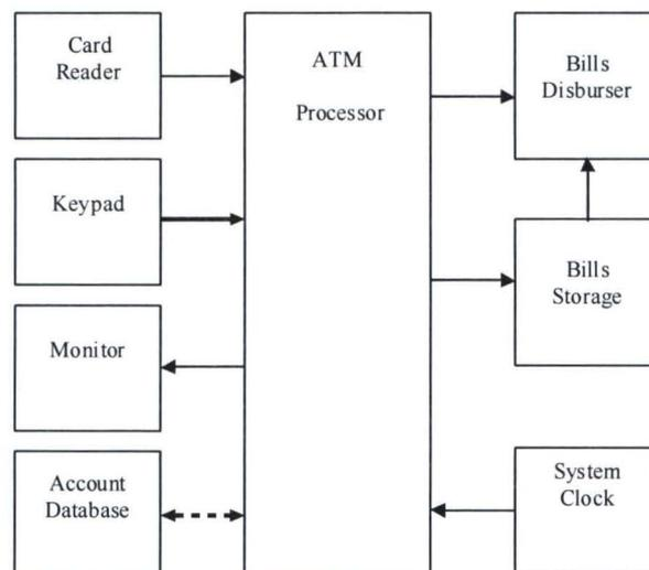
Fig. 3.2 The conceptual model of the ATM system
