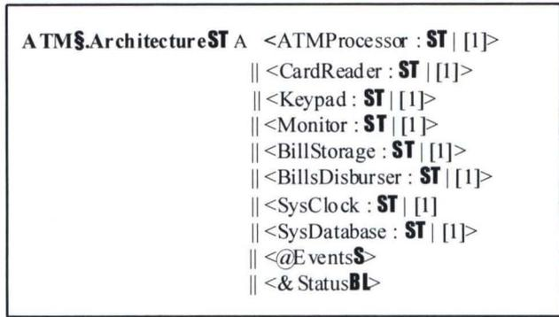
Fig. 3.4 The architectural framework of the ATM system
