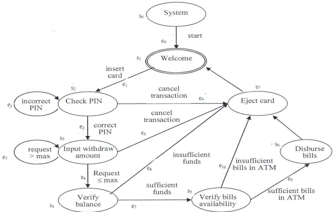
Fig. 3.3 The transition diagram of the ATM behaviors
