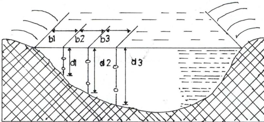
Fig. 1.6.1 View of a stream cross-section showing location of points of observation.
