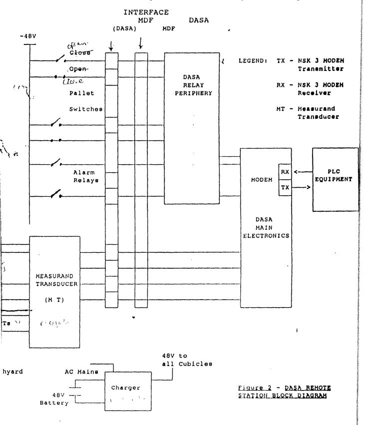
The pallet switches or auxiliary contracts for the CB's or isolator in the switchyard is wired to the MDF. From here, they are taken into DASA Relay periphery via the DASA MDF. The Relay periphery acts to galvanically separate the DASA electronic from the high voltage, high current switchyard. It also act as a memory of the present indication status. Station alarms are also treated similarly as the double indications. These information are sent to DASA main electronics for processing.
