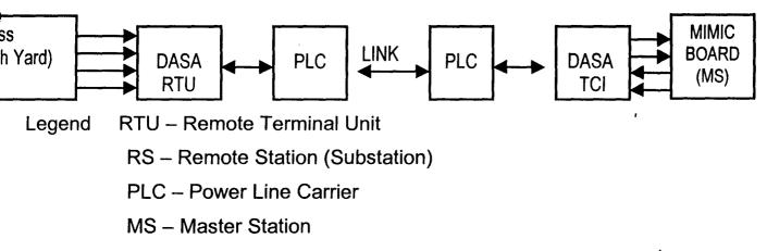
Fig. 1 Block diagram of Shiroro Area Control Centre Scada Scheme.
