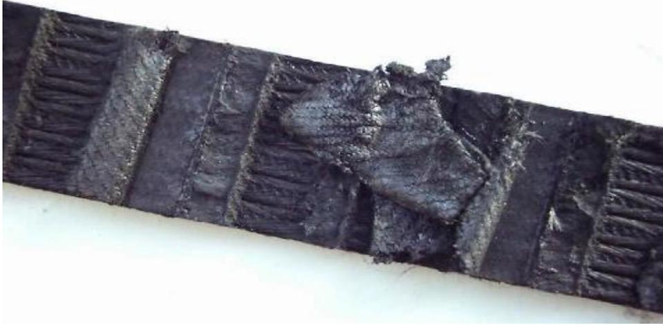
Plate XI: Melting from high temperature operation (Stojanovic, 2011)
