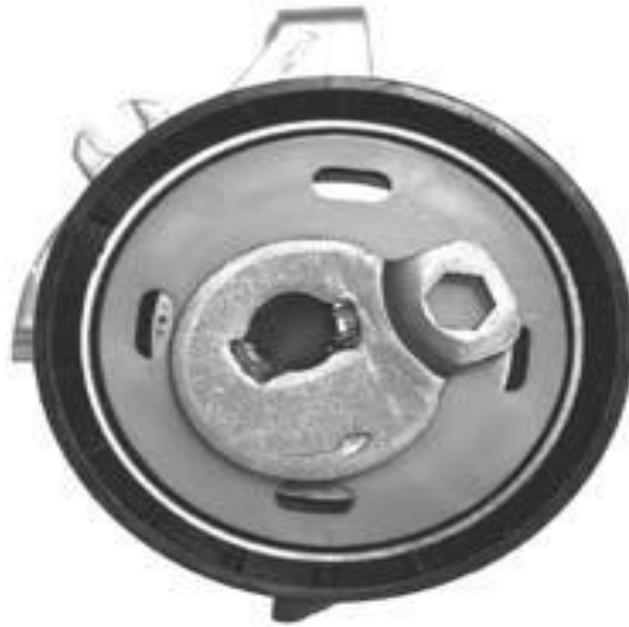
Figure XVI: Automatic Spring-Loaded Tensioner (Auto, 2017)
