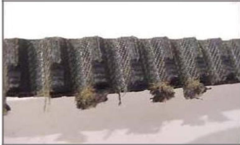
Plate VII: excessive edges wear (Gates, 2010)
