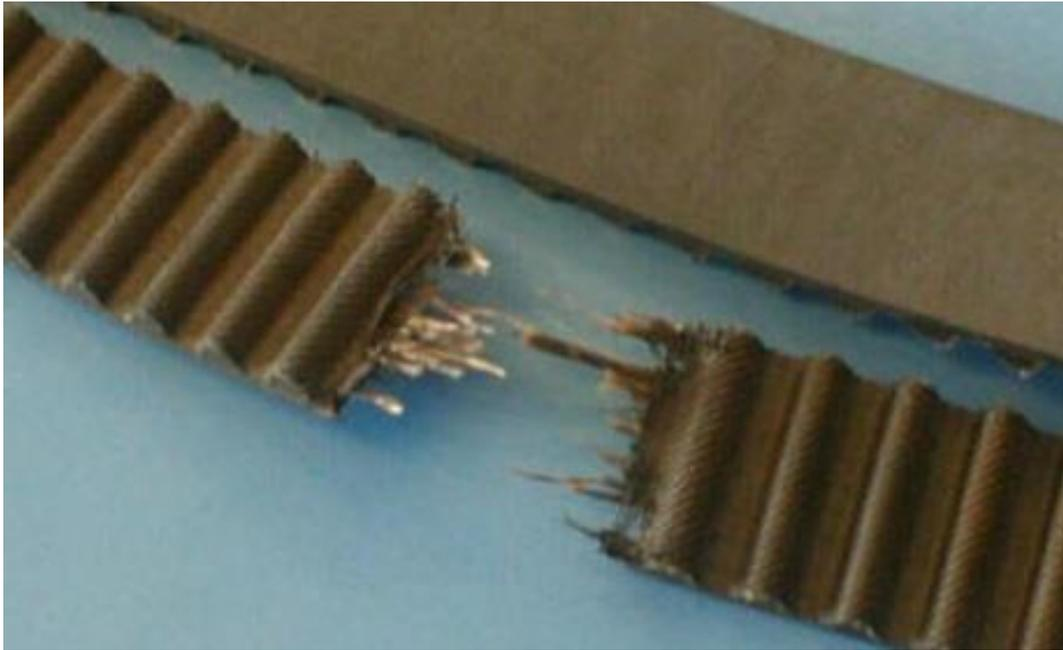
Plate II: Cracking of the drive element
