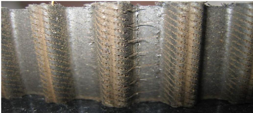
Plate IX: Damage of the face surface of the belt
