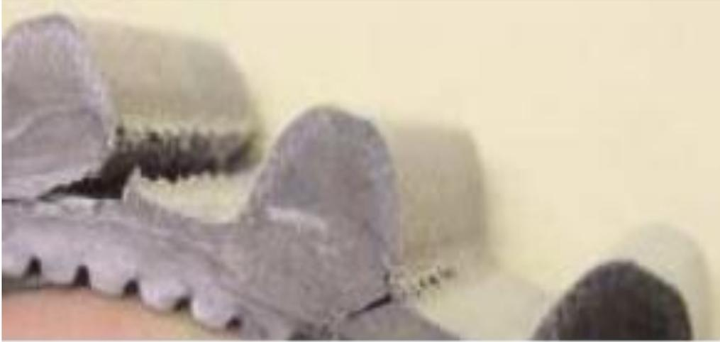
Plate VI: Shear in the belt tooth root ([www.researchgate.net/publication/271705831](http://www.researchgate.net/publication/271705831))
