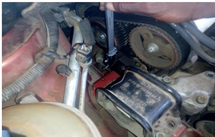
Plate XXV: Measurement of belt Geometry
