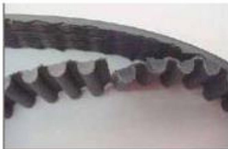
Plate X: Back crack (Stojanovic, 2011)
