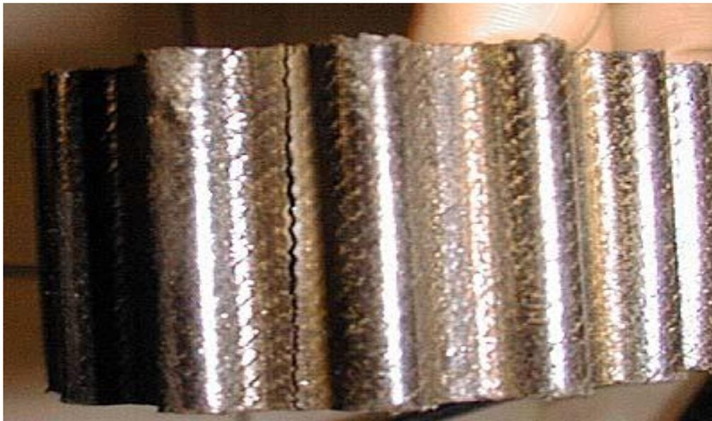
Plate V: Crack in the belt tooth root ([www.researchgate.net/publication/271705831](http://www.researchgate.net/publication/271705831))
