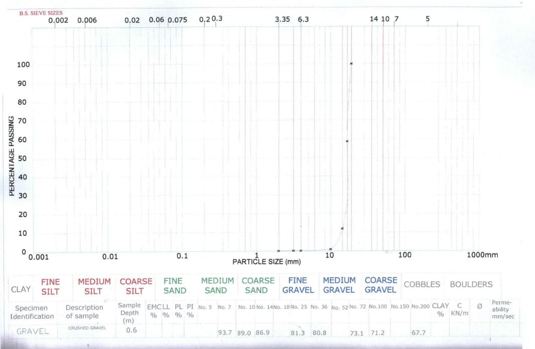
Where D10, D30 and D60 are point where cumulative percentage passing at 10, 30 and 60 cuts the curve on particle size.
