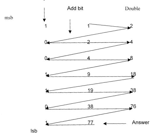
Above is the illustration of binary conversion using the "Double-Dabble" method. Alternatively, this can be carried out as follows:
