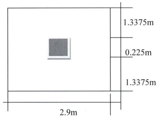
**Fig 4.5.1: Foundation Plan**
