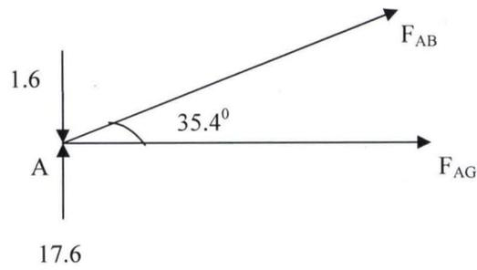
**Fig 4.14: Roof analysis Joint A**
