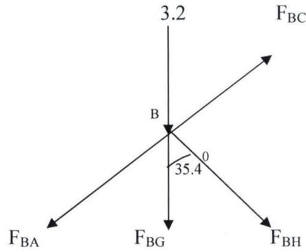
**Fig 4.16: Roof analysis Joint B**
