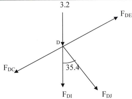
**Fig 4.19.1: Roof analysis Joint D**
