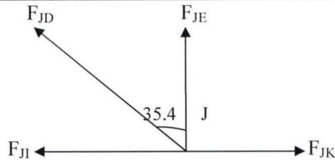
**Fig 4.19.2: Roof analysis Joint J**
