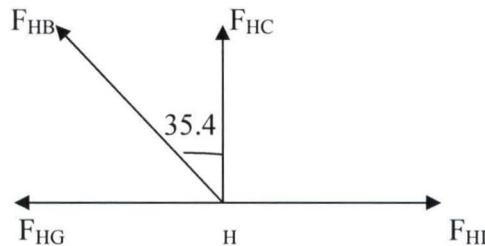
**Fig 4.17: Roof analysis Joint H**
