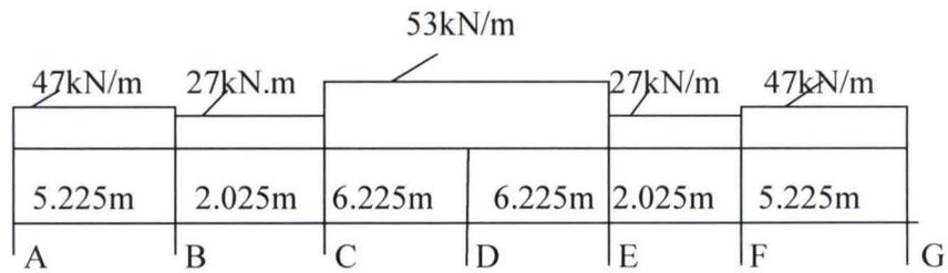
**Figure 4.3.6: BEAM 7****Loadings****Span AB & FG**
