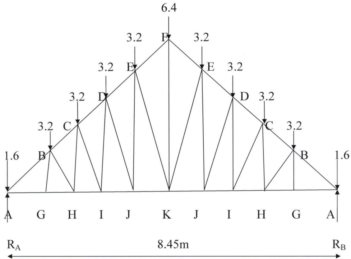
Fig 4.1: Roof Trusses Load Analysis
