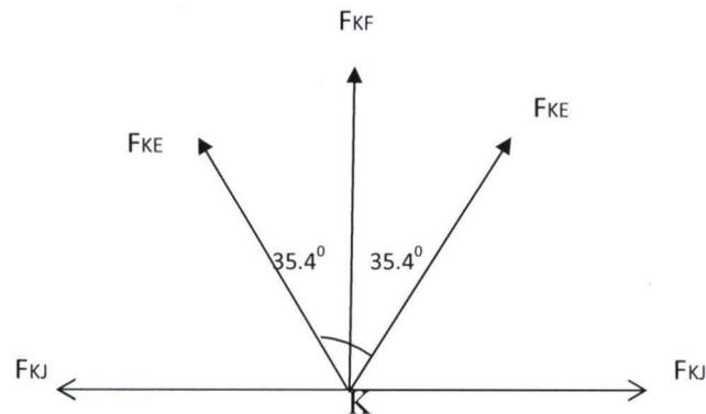
**Fig 4.19.4: Roof analysis Joint K**
