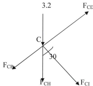
**Fig 4.18: Roof analysis Joint C**
