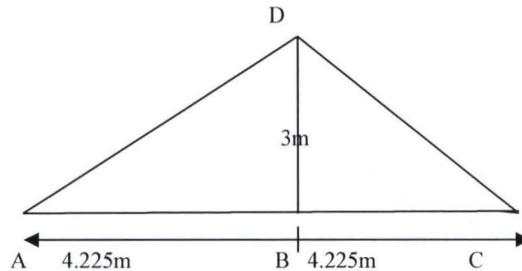
**Fig 4.11: Roof Truss**
