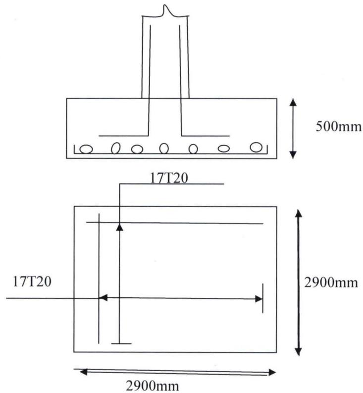
**Fig 4.5.2 Foundation Reinforcement Layout**
